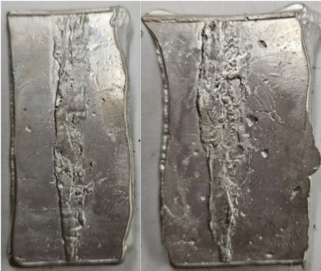
Figure 32: R7 inboard cone spall of Figure 12 with an area of 0.45 in 2 (left) and R7 inboard cone spall of Figure 14 with an area of 0.61 in 2 (right)
