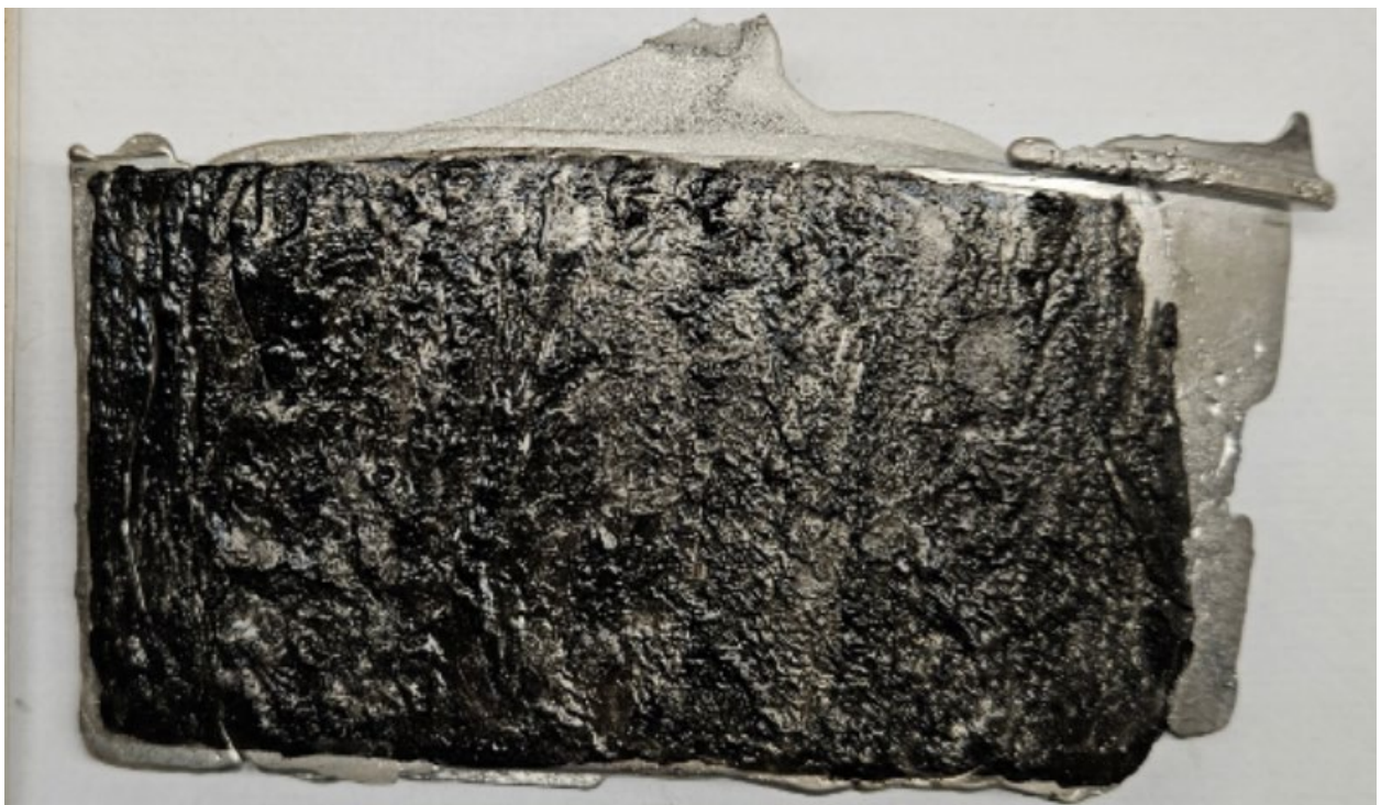
Figure 34: R7 cup outboard raceway spall of Figure 19 with a measured area of 7.88 in 2
