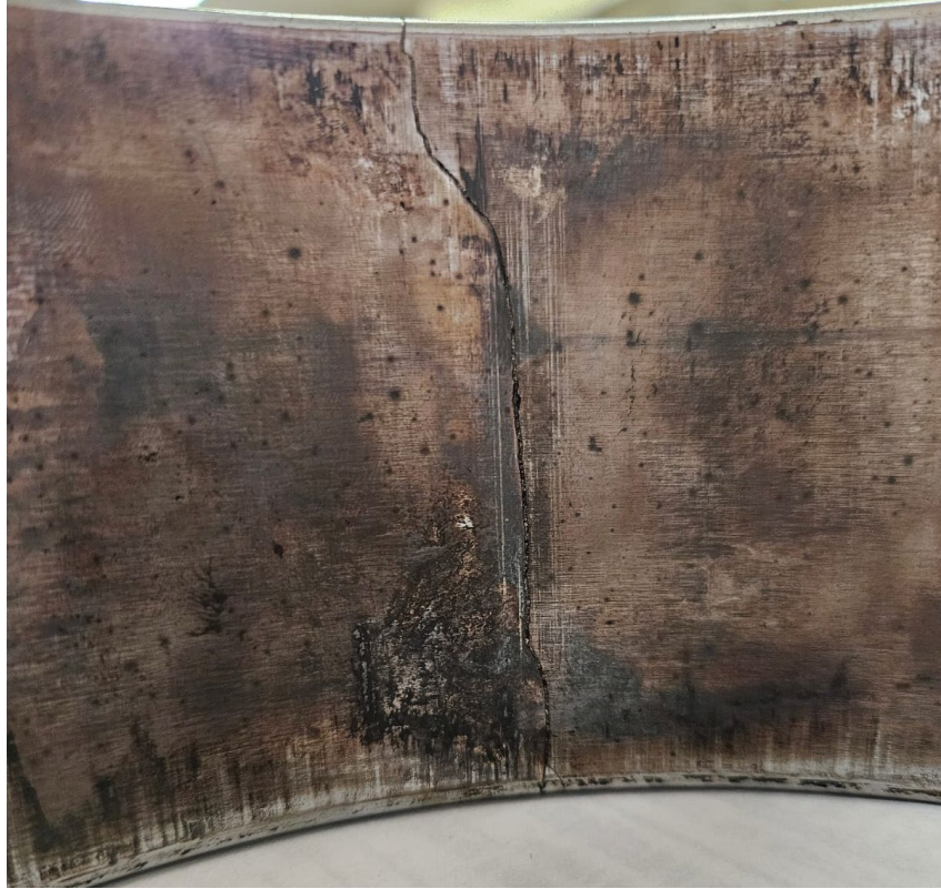
Figure 15: R7 inboard cone (inner ring) raceway with crack spanning its entire width
