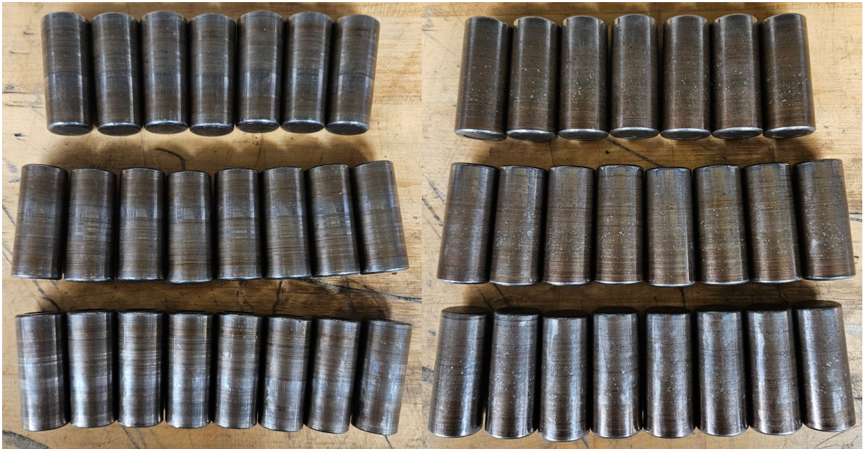
Figure 21: R7 inboard cone rollers (left) and outboard cone rollers (right)
