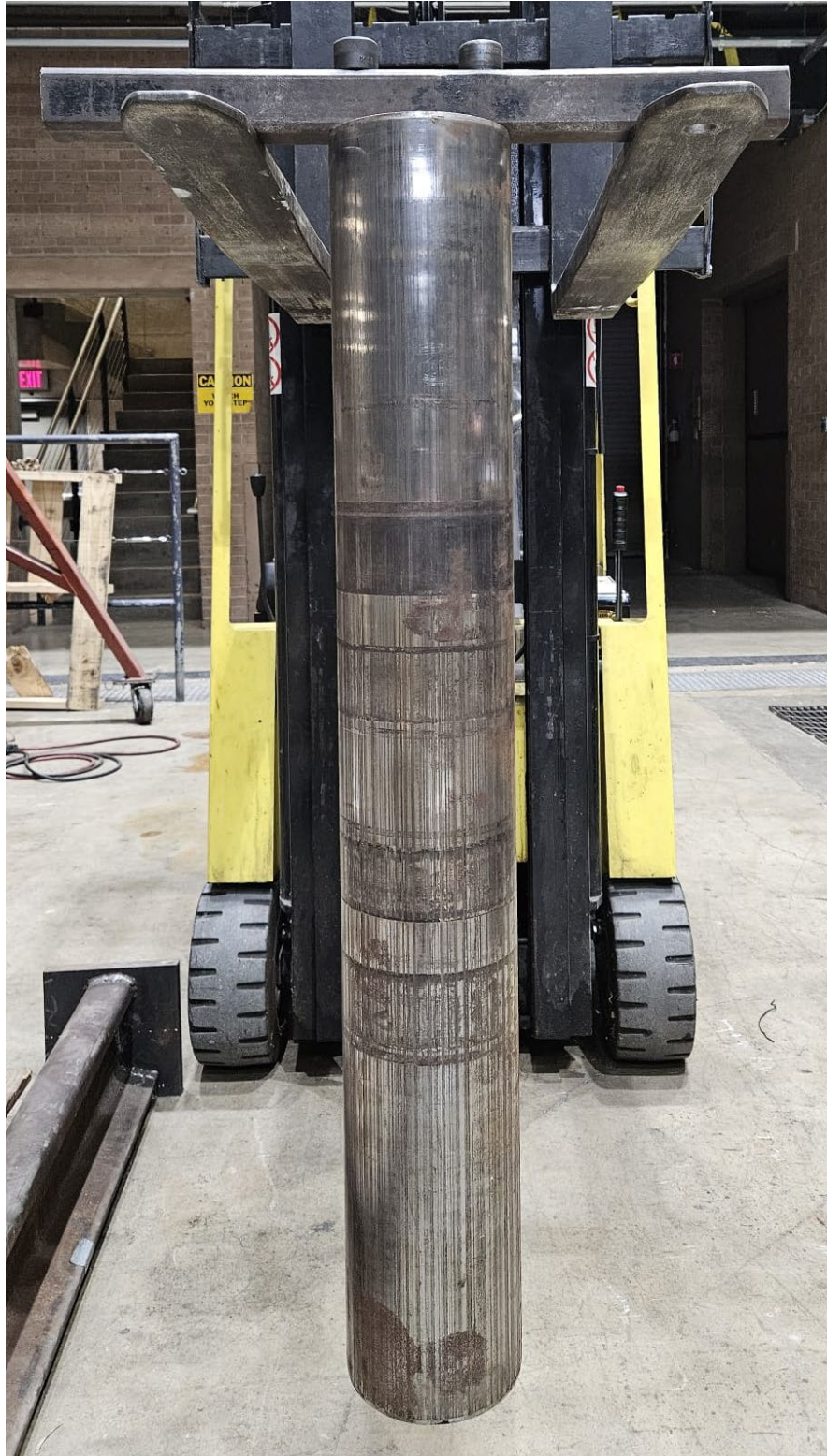
Figure 29: Test axle post press-off showing significant heat tinting in the location where the R7 inboard cone assembly was positioned
