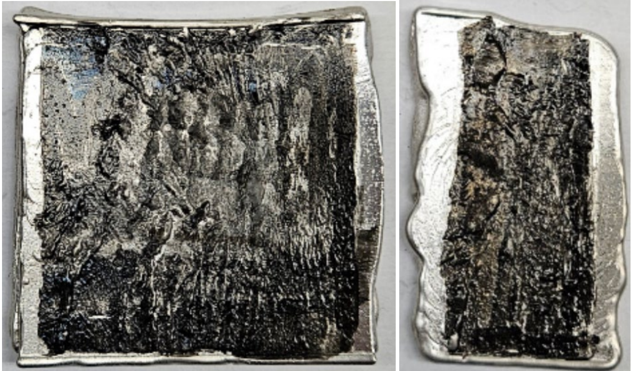
Figure 33: R7 outboard cone spall of Figure 17 with a measured area of 2.47 in 2 (left) and R7 outboard cone spall of Figure 18 with a measured area of 1.43 in 2 (right)
