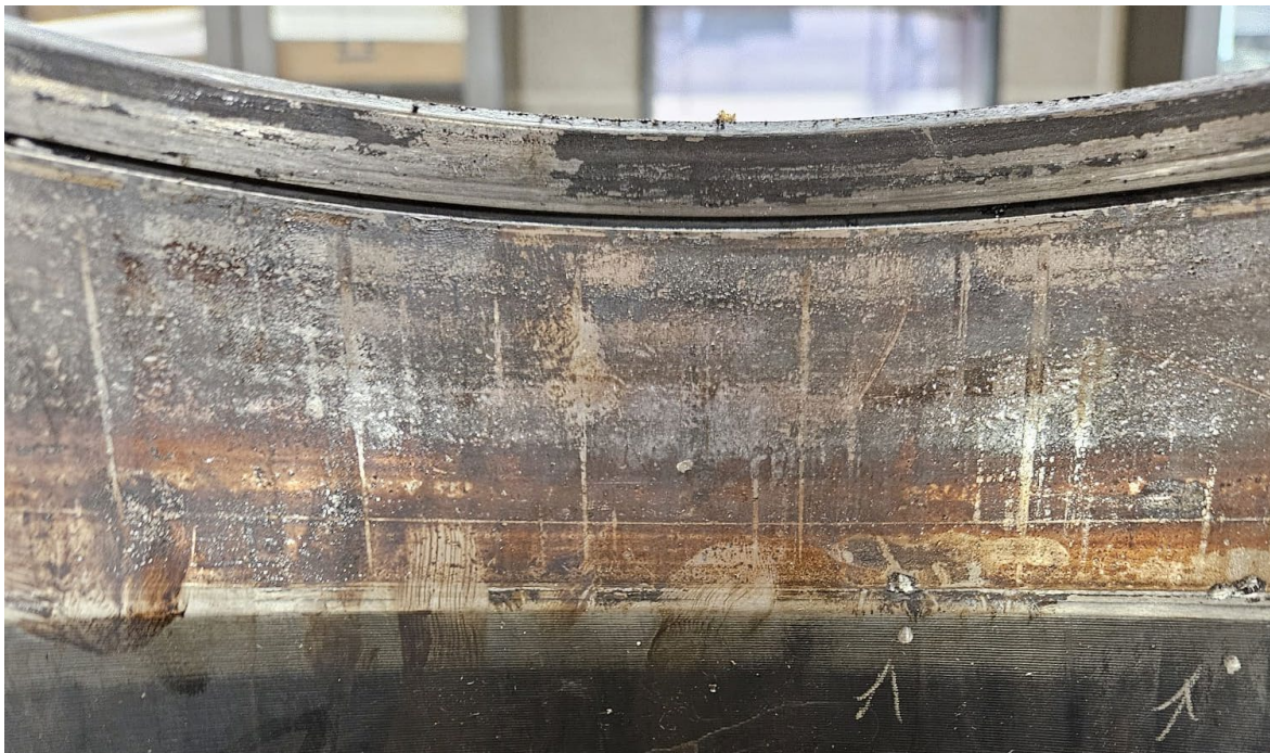
Figure 20: R7 cup (outer ring) inboard raceway on loaded side showing repaired spalls
