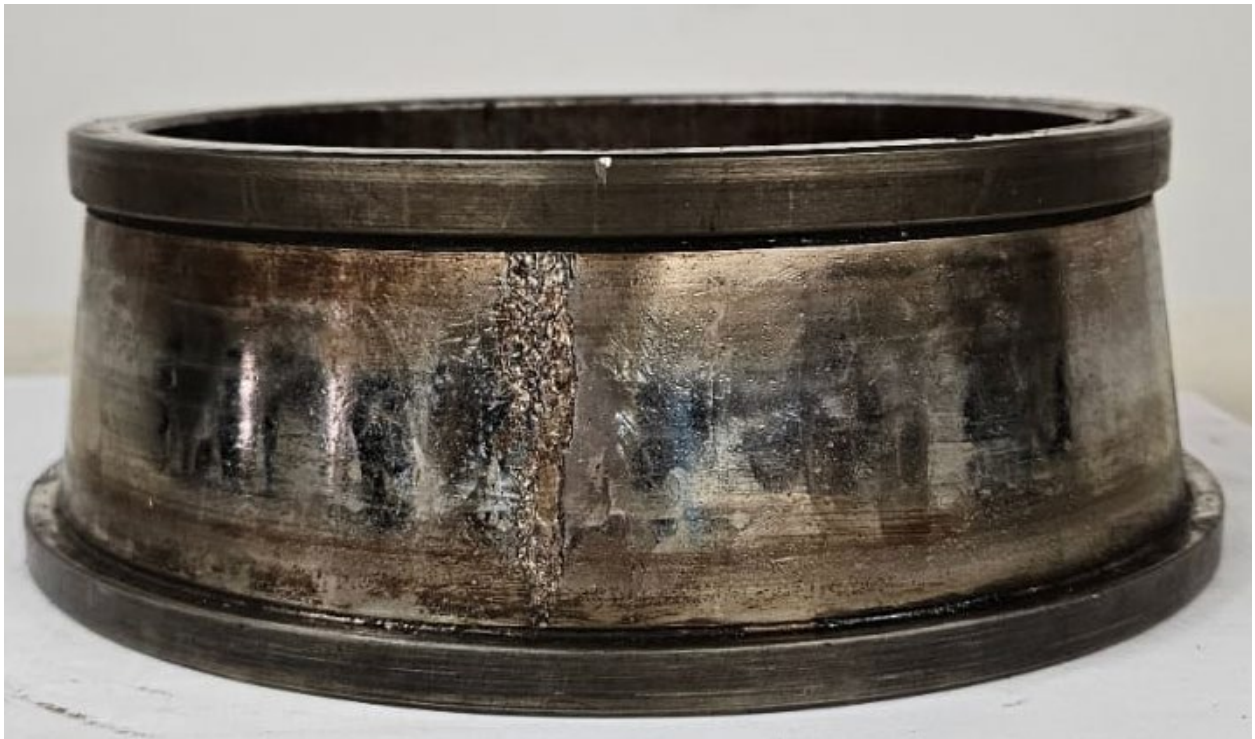
Figure 14: R7 inboard cone (inner ring) raceway – Picture 4
