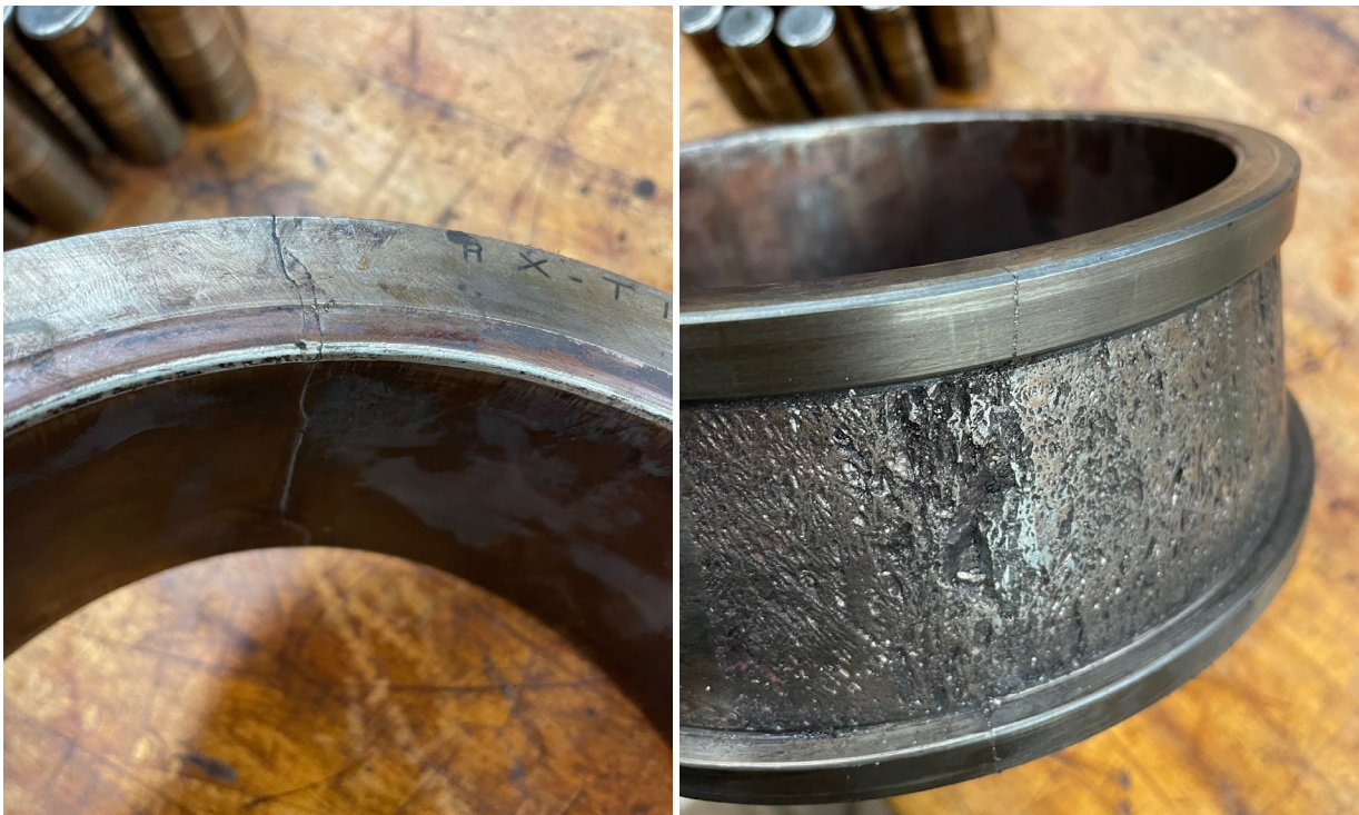
Figure 16: R7 inboard cone (inner ring) raceway showing crack along the width
