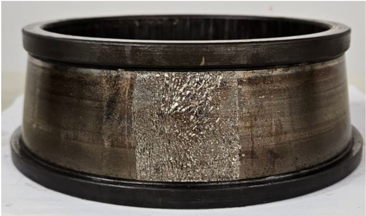
Figure 17: R7 outboard cone (inner ring) raceway – Picture 1
