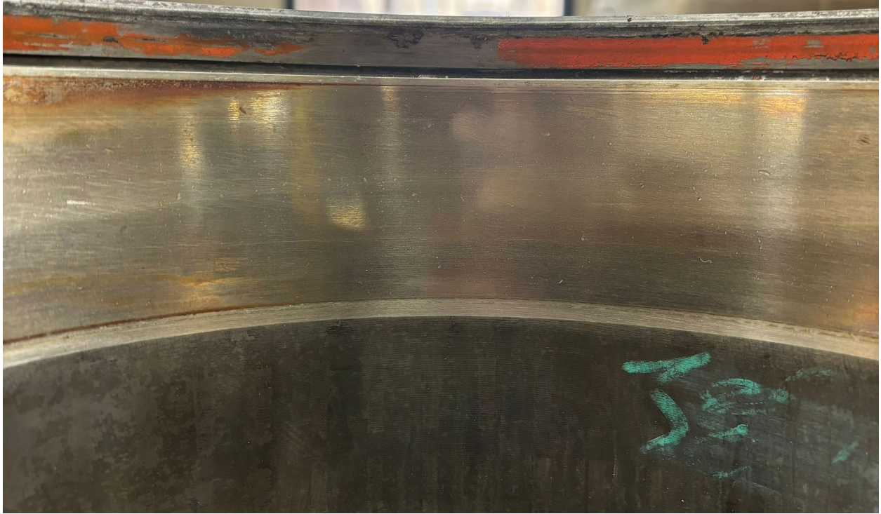
Figure 27: L7 cup (outer ring) outboard raceway on loaded side
