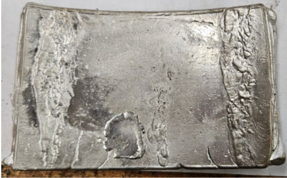
Figure 31: R7 inboard cone spall of Figure 13 with a measured area of 1.82 in 2
