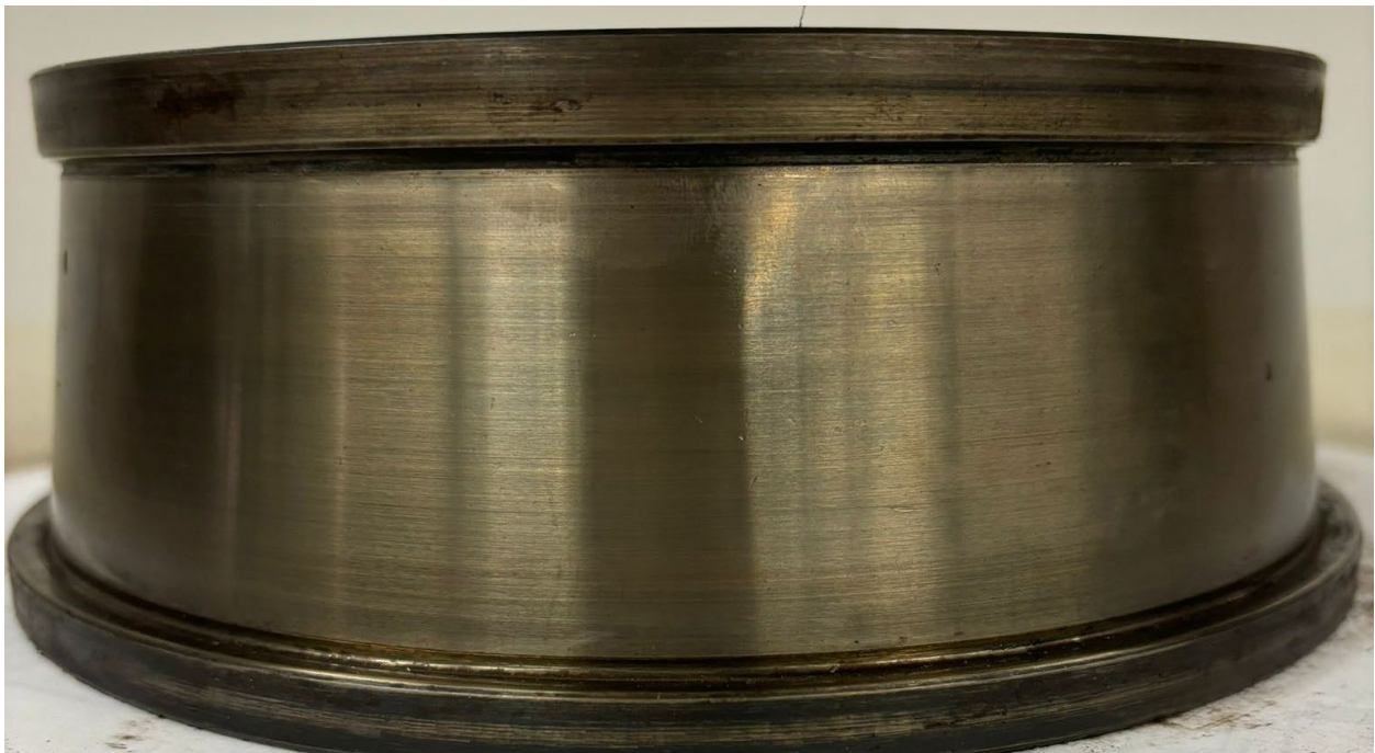
Figure 22: L7 inboard cone raceway
