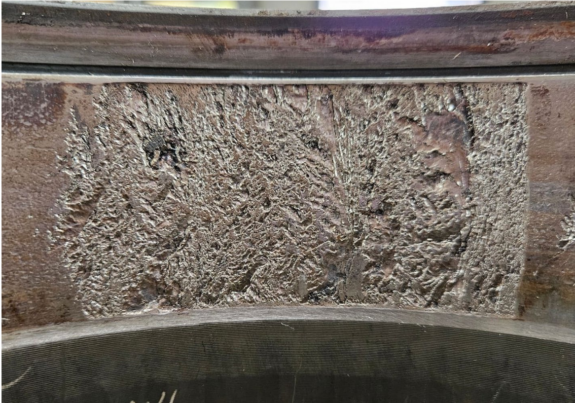
Figure 19: R7 cup (outer ring) outboard raceway damage on loaded side
