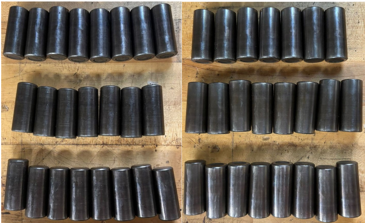
Figure 28: L7 inboard cone rollers (left) and outboard cone rollers (right)
