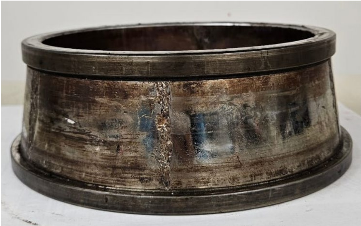
Figure 12: R7 inboard cone (inner ring) raceway – Picture 2
