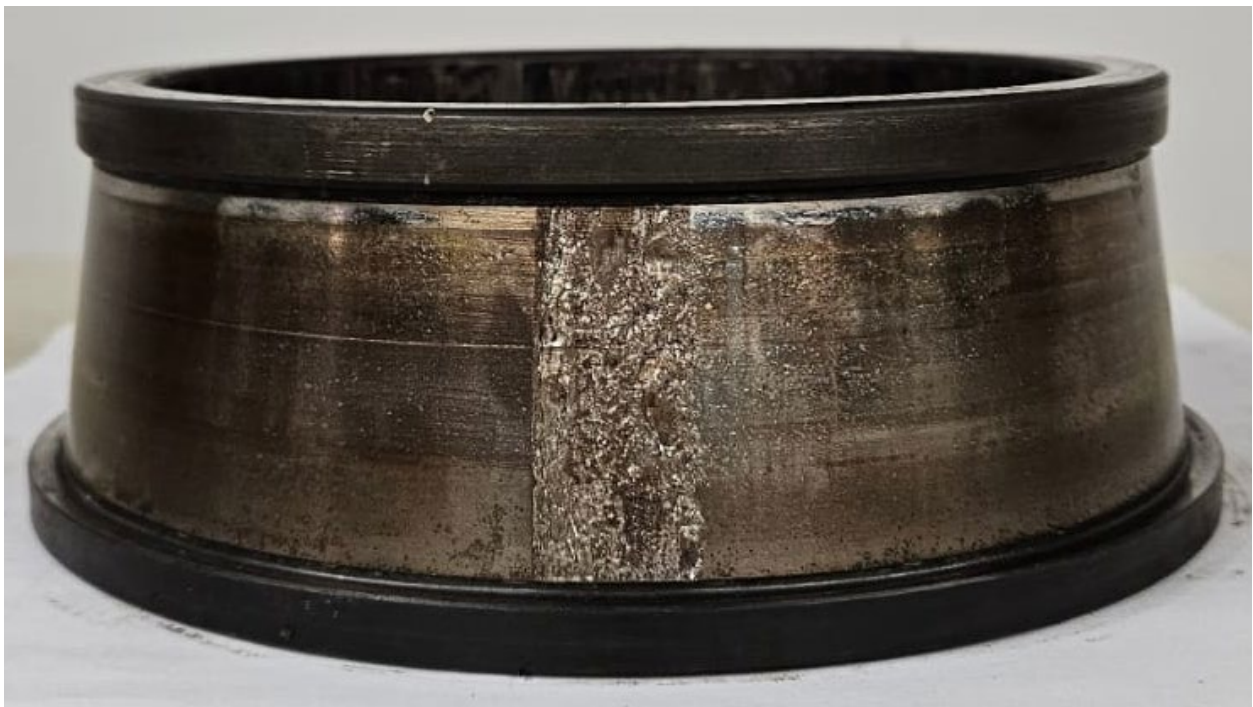
Figure 18: R7 outboard cone (inner ring) raceway – Picture 2
