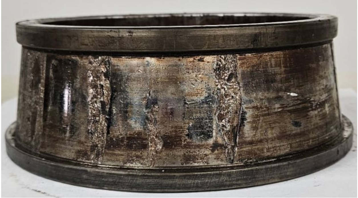
Figure 13: R7 inboard cone (inner ring) raceway – Picture 3
