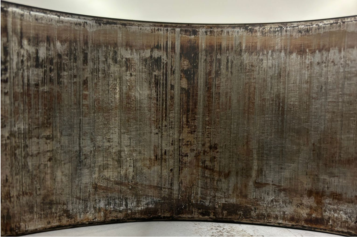
Figure 23: L7 inboard cone raceway inner diameter surface which is pressed on test axle
