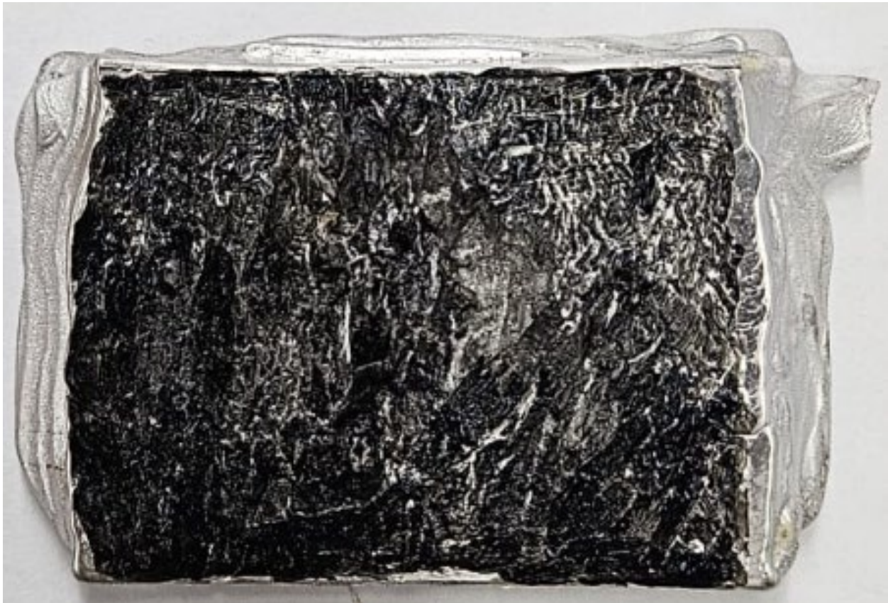
Figure 30: One of three parts of the R7 inboard cone spall which had a total area of 13.6 in 2 (refer to Figure 11)
