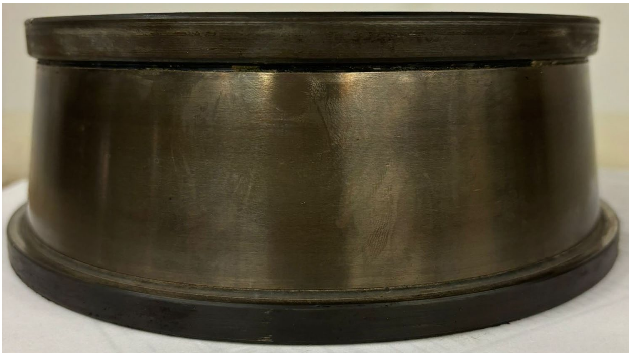
Figure 24: L7 outboard cone raceway
