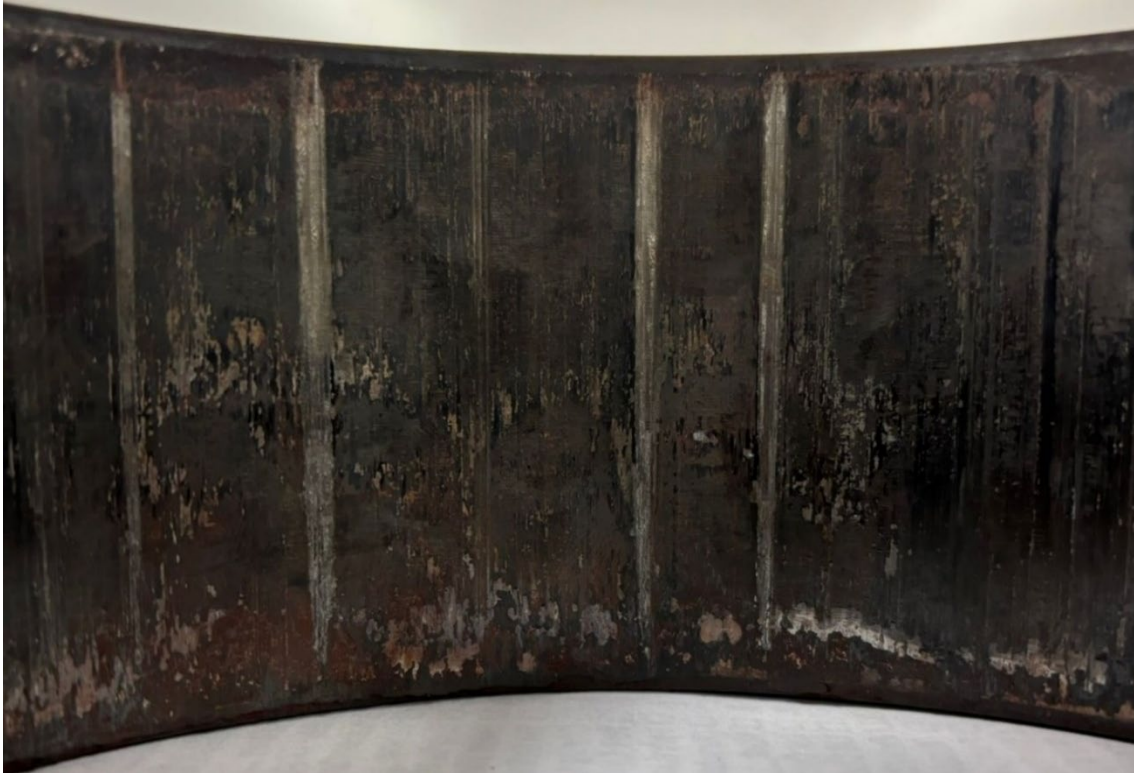
Figure 25: L7 outboard cone raceway inner diameter surface which is pressed on test axle
