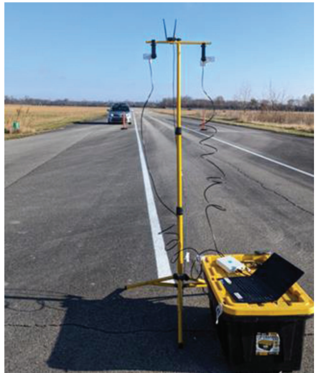
Figure 5.6 Capture of the communication test with static vehicle.
