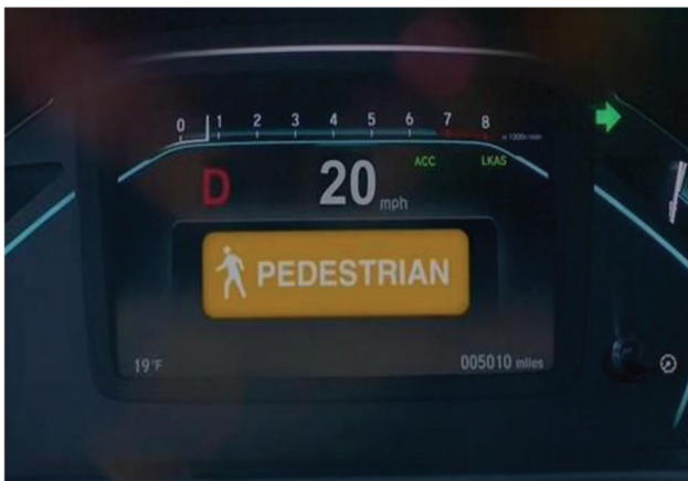
Figure 2.3 Pedestrian scenario from Honda and Verizon’s collaboration: pedestrian warning shown on the dashboard.
