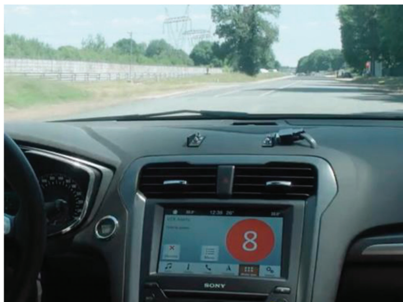
Figure 2.4 Use case of signal phase shown from 5GAA demonstration.
