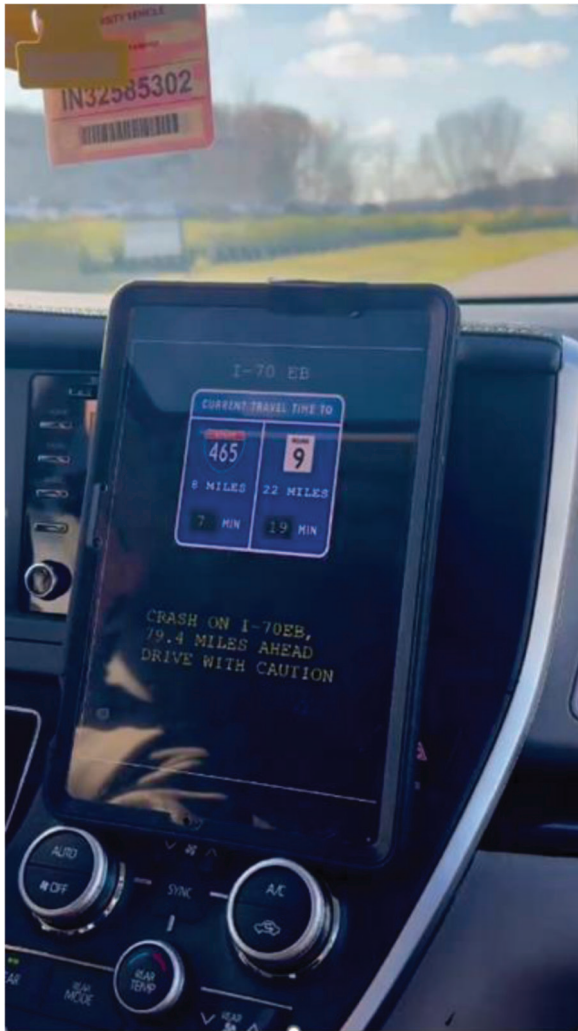
Figure 3.4 RampCast GUI shown in a driving scenario using a tablet.
