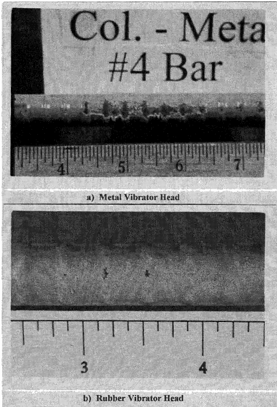
Figure 2. 19 Vibration damage to epoxy coating
