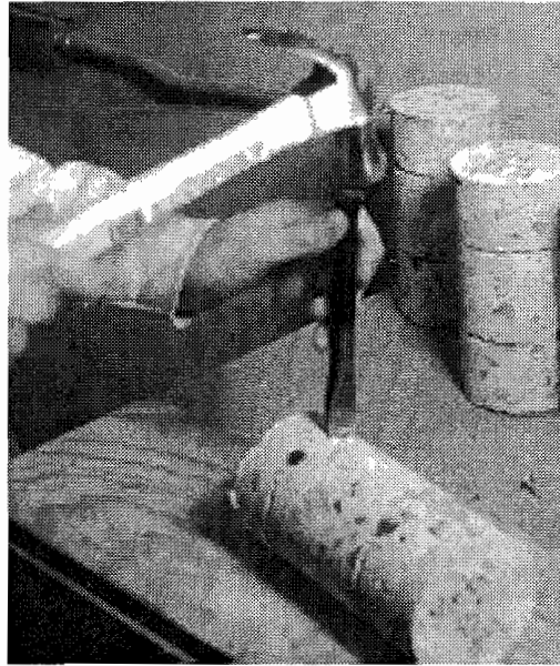
Figure 4. 17 Splitting cores at level of reinforcement
