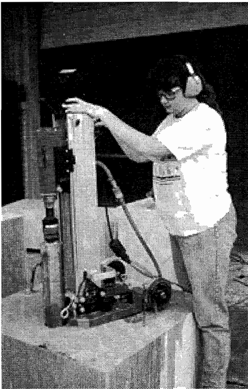
Figure 4.13 Coring reinforced concrete test specimen
