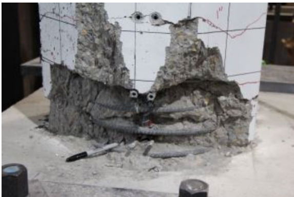
(c) At the end of test (cracks, spalling, concrete delamination, and fractured rebar)
