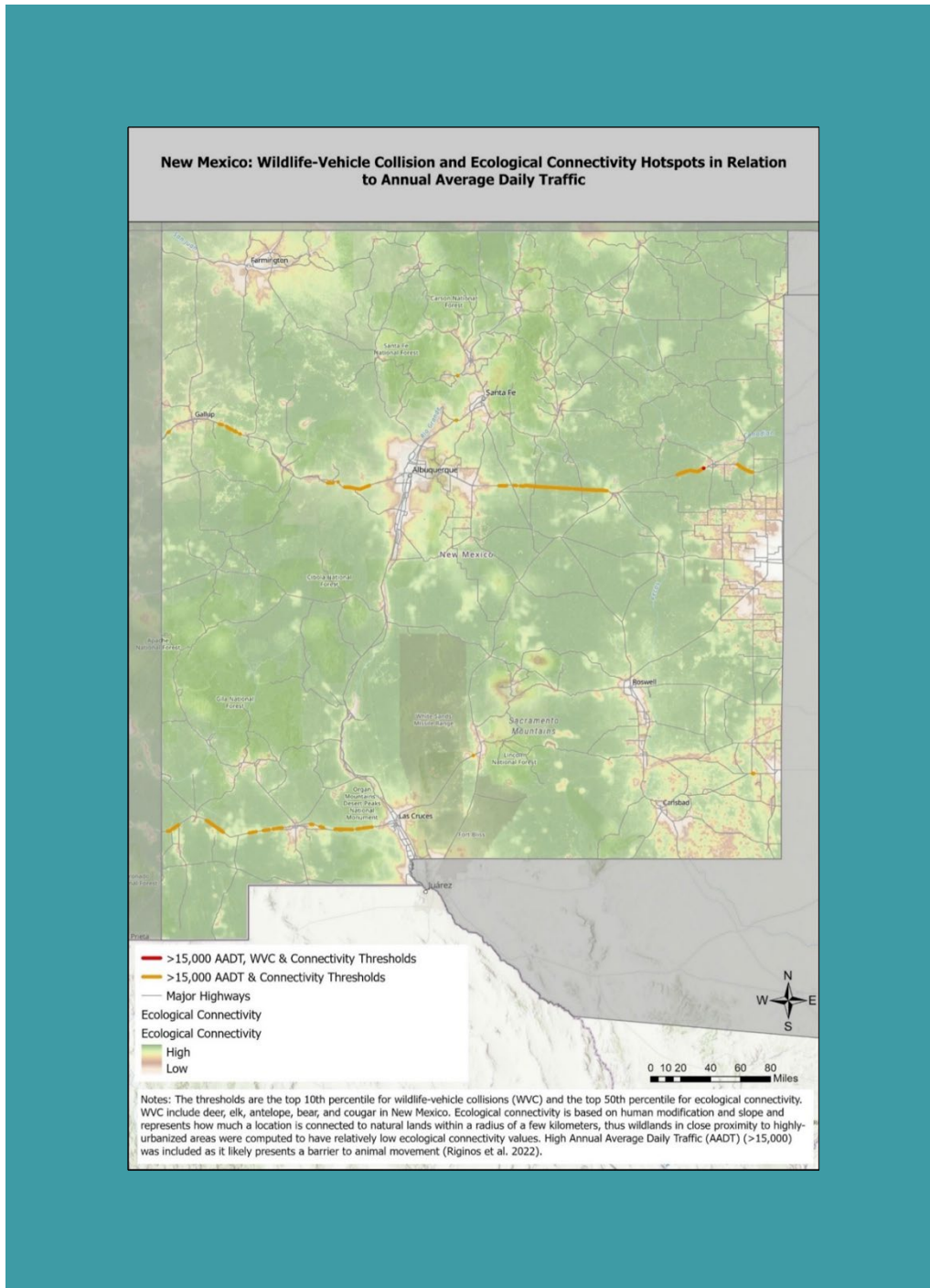
Figure 39. Road segments i) above the top 10 th percentile for WVCs and the 50 th percentile for ecological connectivity, with high traffic volume of AADT \geq 15,000 (red), and ii) above the 50 th percentile for ecological connectivity with high traffic volume of AADT \geq 15,000 (orange).
