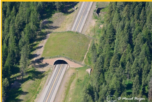
Figure 1. Examples of a wildlife underpass with fencing and nearby jump-out, and of a wildlife overpass, both along US Hwy 93, Flathead Indian Reservation, Montana, USA
