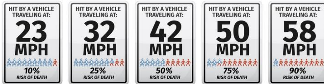
Figure 13 Likelihood of Fatality at Different Speeds of Pedestrian & Vehicle Crashes. Source: National Roadway Safety Strategy https://www.transportation.gov/NRSS/SaferSpeeds
