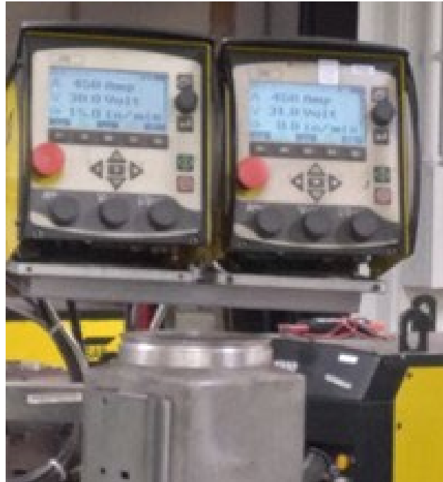
Figure 11.1 ESAB SAW equipment
