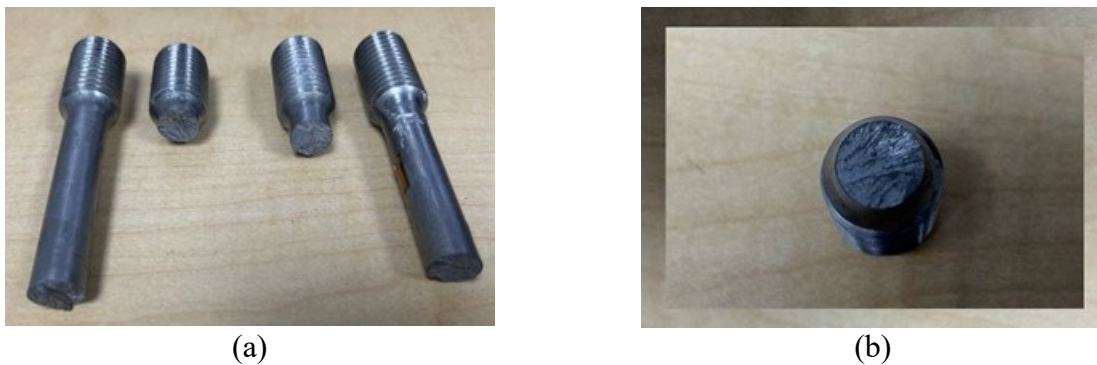
Figure 10.13 Failure shapes of the weld area samples
