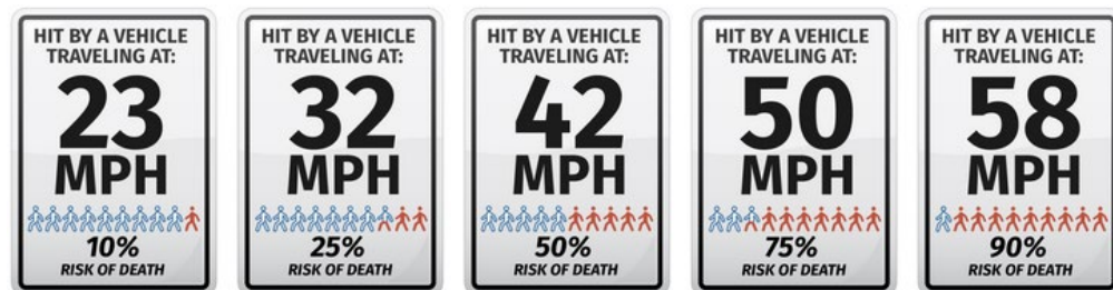
Figure 6 Likelihood of Fatality at Different Speeds of Pedestrian & Vehicle Crashes. Source: National Roadway Safety Strategy https://www.transportation.gov/NRSS/SaferSpeeds
