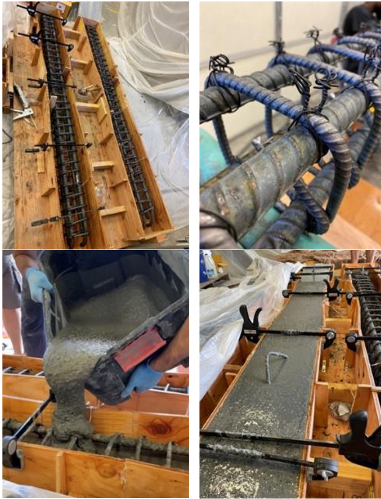
Figure 6.5 Fabrication of UHPC tie specimen
