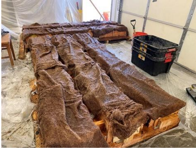
Figure 6.6 Curing of UHPC tie specimens using moist burlap
