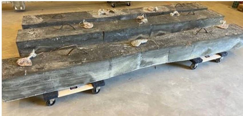
Figure 6.7 UHPC tie specimens after removed from formwork
