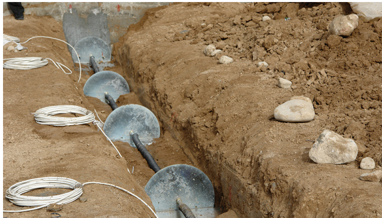
Figure 4: Slope Extensometers used to measure strains in a large area ( https://sisgeo.com/ ).
