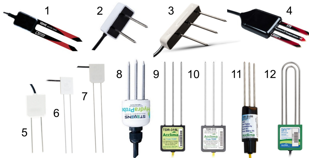
Figure 6: Different types of commercial soil moisture sensors(Ferrarezi, Nogueira, and Zepeda 2020).
