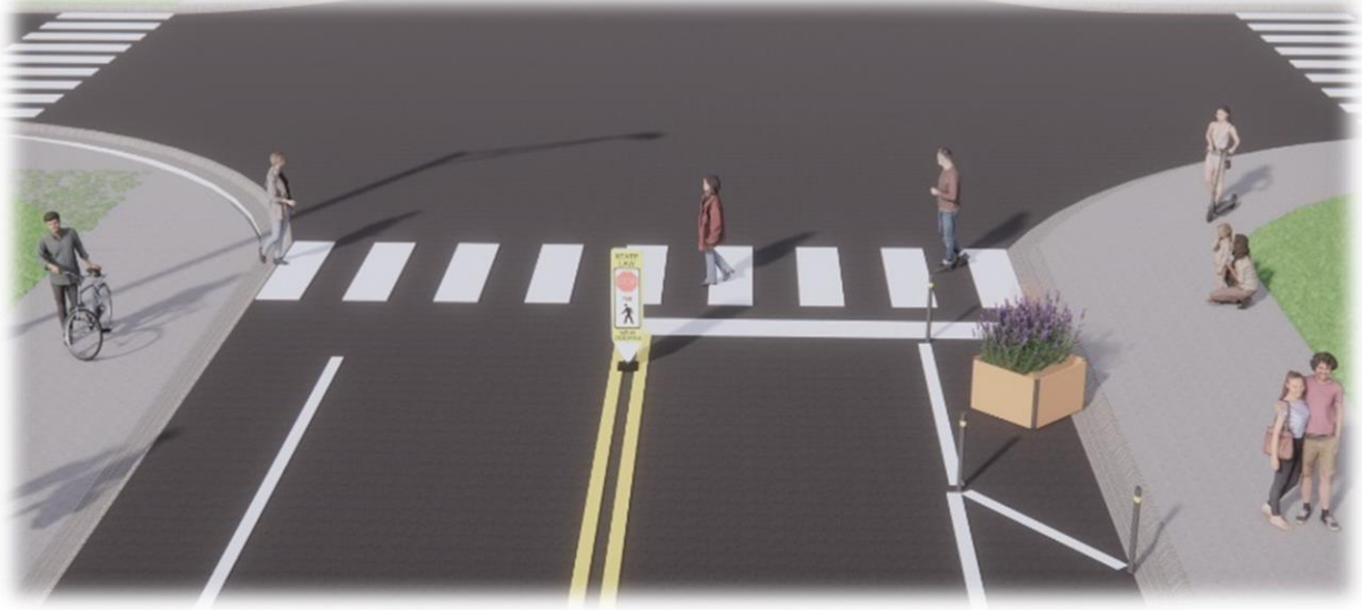
Figure 17. Proposed curb extension at Ousel Falls Rd & Aspen Leaf.
