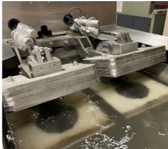
Figure 3.8 Photographic view of the submerged HWT specimens at 50^{\circ}\text{C} subjected to wheel loading
