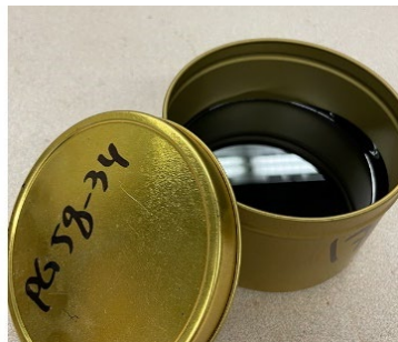
Figure 3.2 A photographic view of the PG 58-34 asphalt binder sample in a small can
