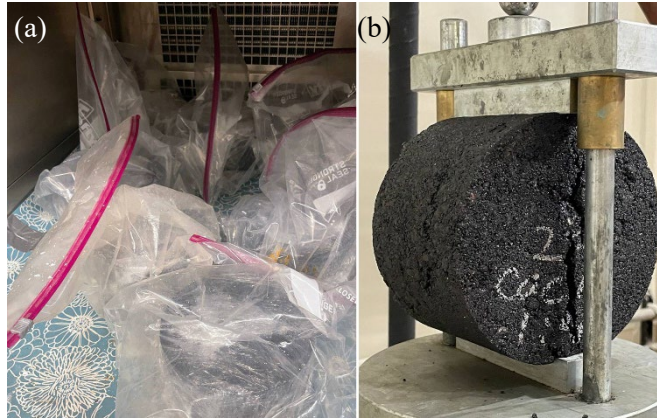
Figure 3.7 Photographic views of (a) TSR specimens in the environmental chamber, (b) a TSR specimen during testing
