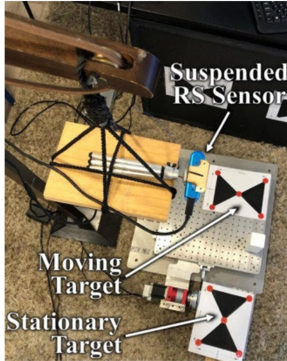
Figure 3.1 Overview of non-stationary 2C planar measurement set-up
