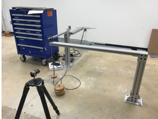
Figure 3. Experimental test frame with camera and laser displacement sensor.
