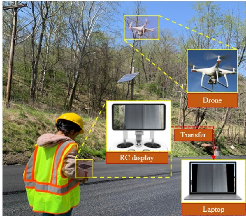
Figure 5. Overview of proposed setup of the UAV used for tack coat uniformity inspection.
