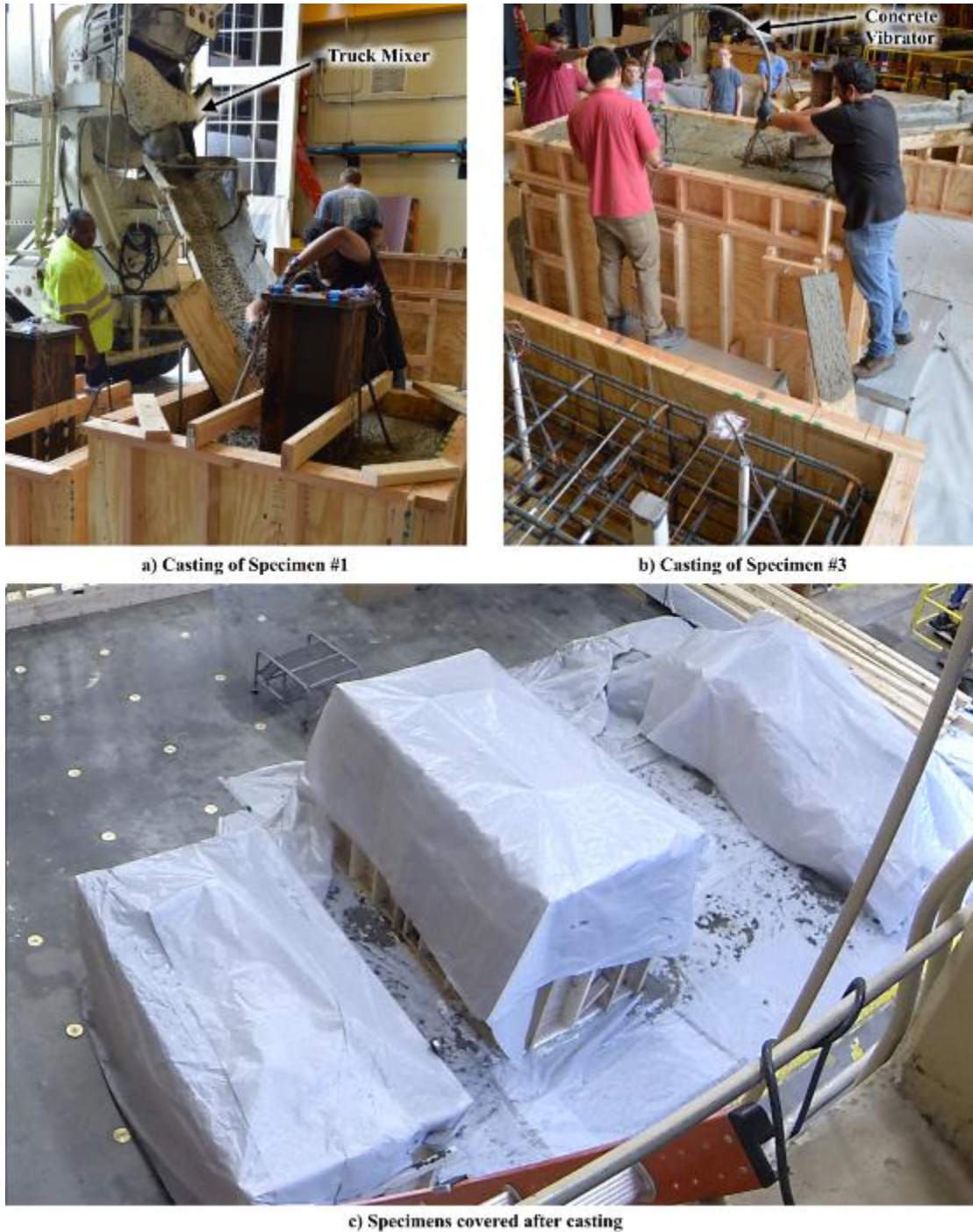
Figure 5-6 Figure showing details of concrete casting
