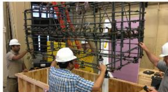
c) Rebar cage being lowered into Specimen #4
