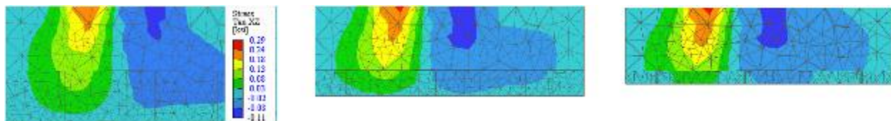
Figure 4-16 Figure comparing shear stresses in foundation for different embedment depths
