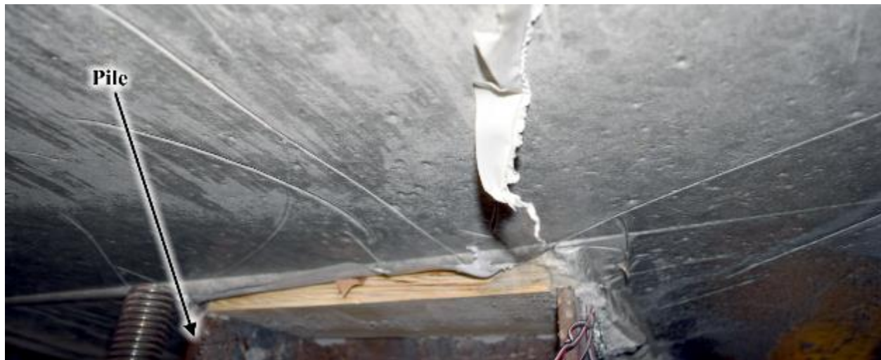
Figure 6-11 Figures showing no visible damage to the concrete surrounding the pile in Specimen #3
