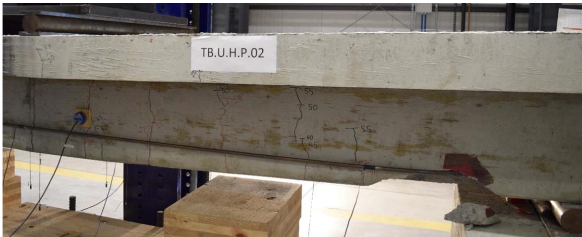
Figure 7-17 Anchorage failure of Specimen TB.U.H.P.02
