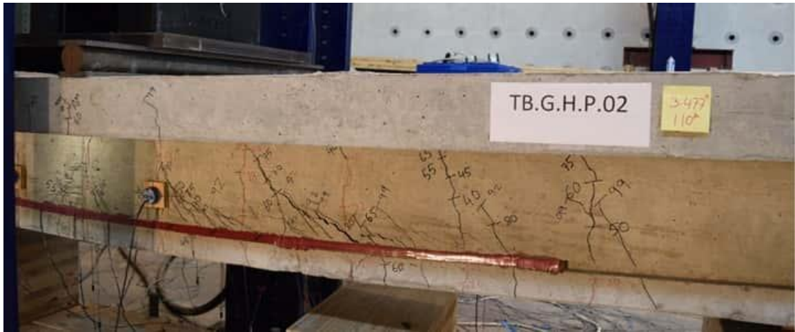
Figure 7-4 Concrete-epoxy interface failure for Specimen TB.G.H.P.02
