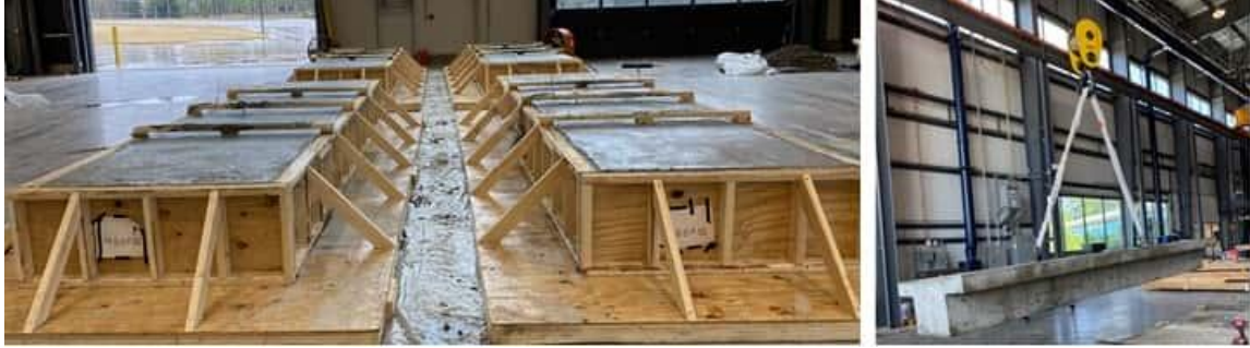
Figure 6-5 Specimen after casting (Left) and Lifting of the specimen (Right)
