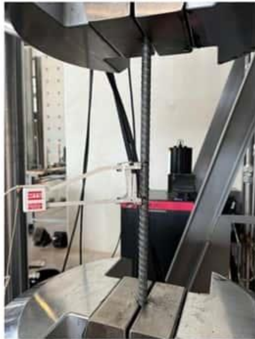
Figure 3-2 Tensile test of #4 reinforcing steel
