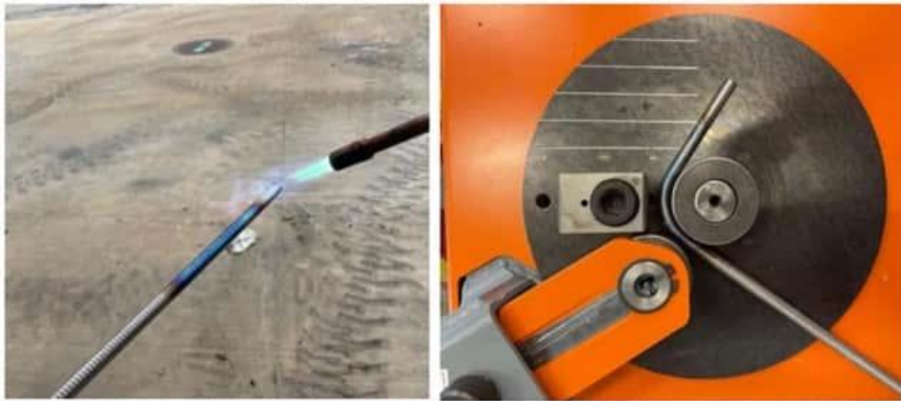
Figure 4-13 TiAB heating (heating) and bending (right)
