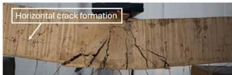
Figure 5-16 Horizontal crack formation in the shear span of SB96
