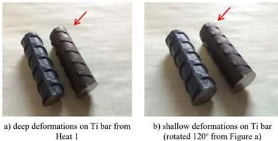
Figure 2-8 ASTM A615 #5 bar (left) and titanium bar (right, with red arrow) (Platt and Harries, 2018a)
