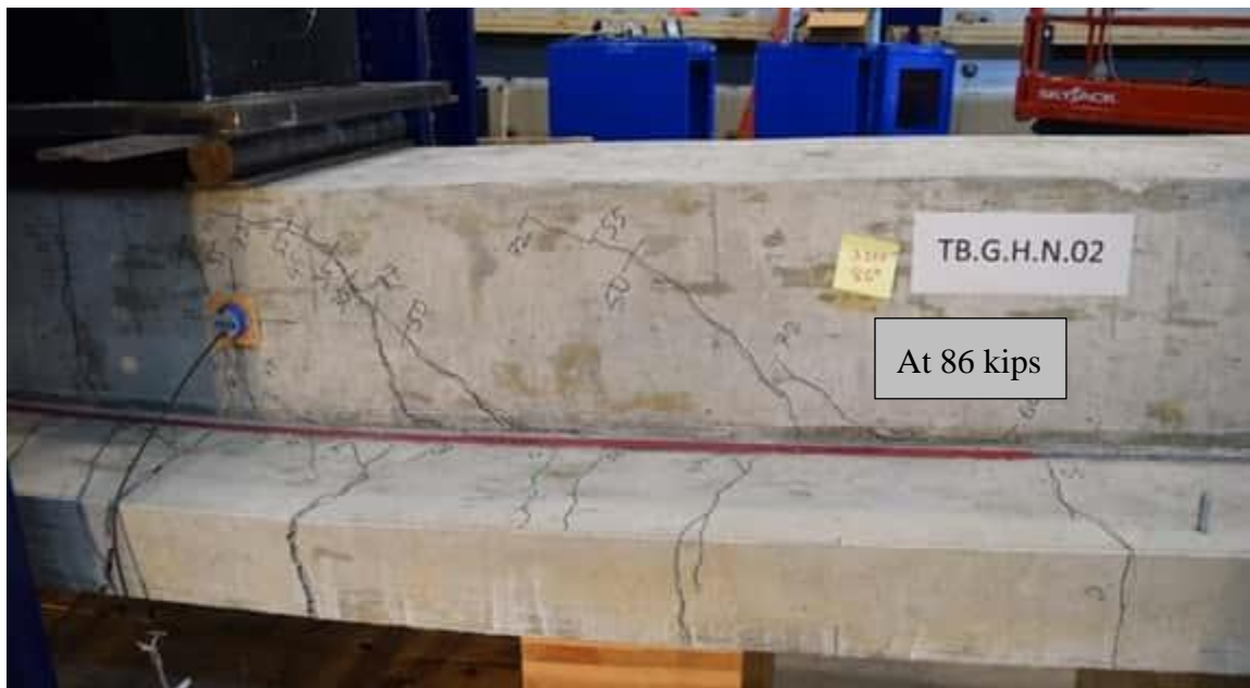
Figure 7-7 Cracking in Specimen TB.G.H.N.02 at 86 kips
