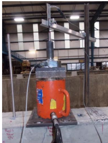
Figure 2-5 Pull-out test setup for TiAB (Barker 2014)
