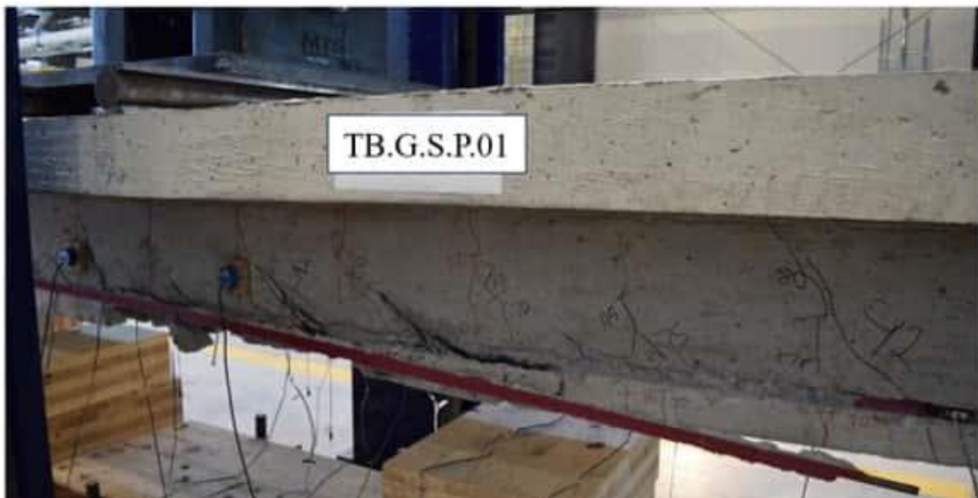
Figure 7-10 Concrete-epoxy interface failure for Specimen TB.G.S.P.01 at 100 kips
