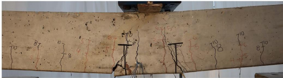
b) Widened inclined cracks at 13.8 kips
