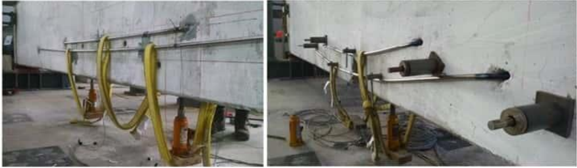
Figure 2-15 Epoxy Anchors (left) and Prestressing Chuck Anchors (right) (Vavra, 2016)
