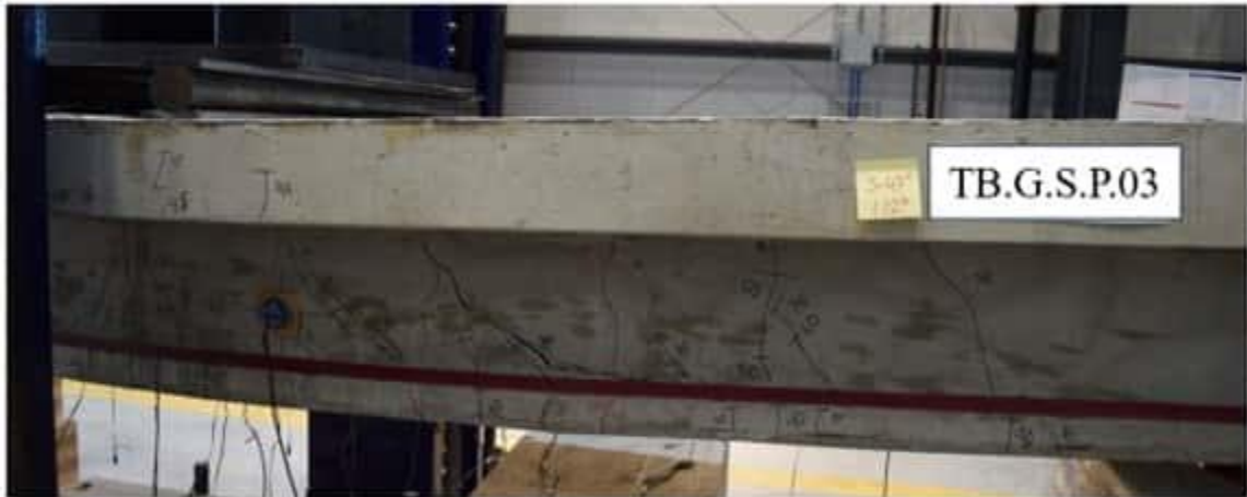
Figure 7-12 Concrete-epoxy interface failure for Specimen TB.G.S.P.03 at 112 kips load
