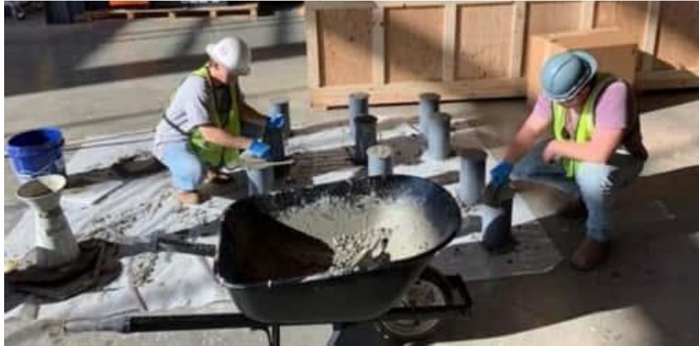
Figure 4-7 Cylinder preparation for strength evaluation
