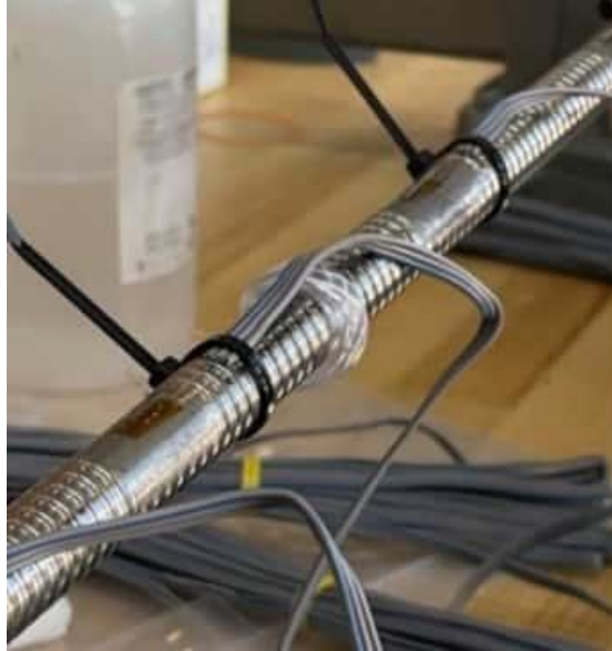
Figure 4-14 TiAB with wedge and strain gauges
