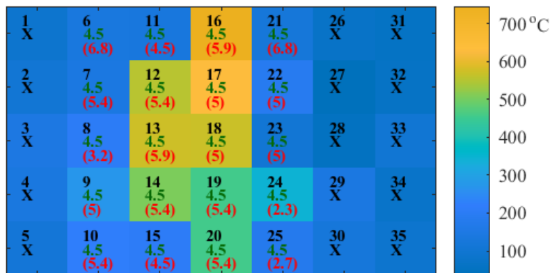
Figure 7.7 Pre-fire and post-fire abrasion resistance results. The change in weights overlaid on the surface temperature map (green values are pre-fire weight changes and red values are post-fire weight changes. “X” indicates areas where no cores were taken) (units are grams).
