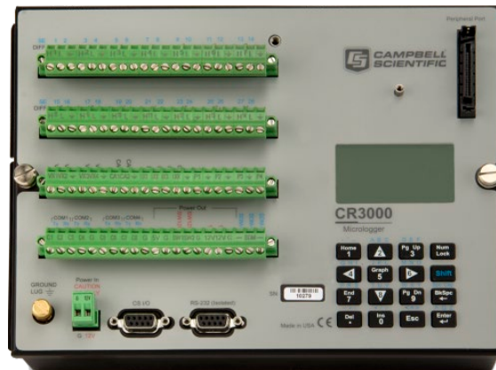
Figure 3.7 CR3000 Data Acquisition System
