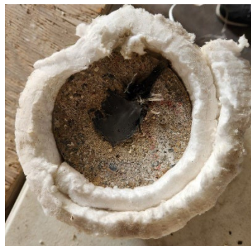
Figure 7.6 A core sample with PC overlay insulated before exposing to heat in a furnace
