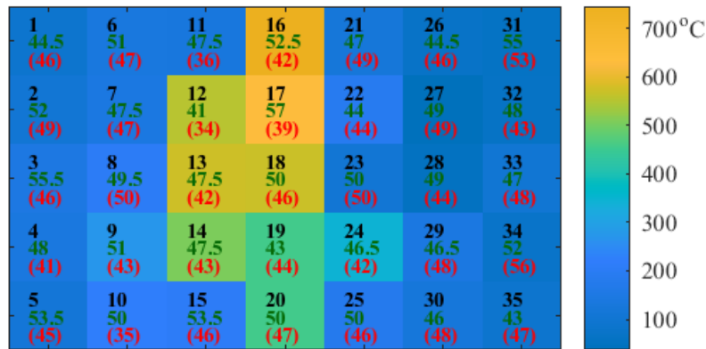
Figure 7.2 Pre-fire and post-fire surface hardness results (green values are pre-fire surface hardness and red values are post-fire surface hardness)
