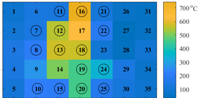
Figure 7.5 Failure mode in bond strength test (colors represent the maximum recorded temperatures, and the circles around numbers represent locations with bond failure).
