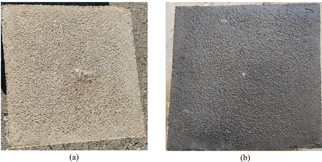
Figure 8.1 Test slabs a) control slab without intumescent layer and b) slab with intumescent layer applied
