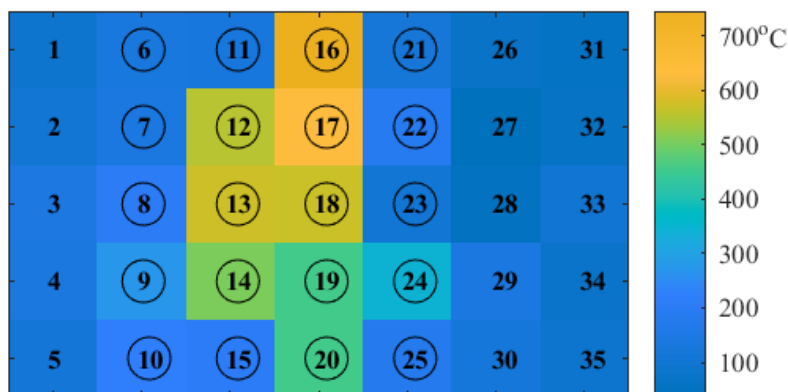
Figure 6.7 Maximum recorded temperature at different locations over the surface (circles shows the locations for post-fire test sampling)
