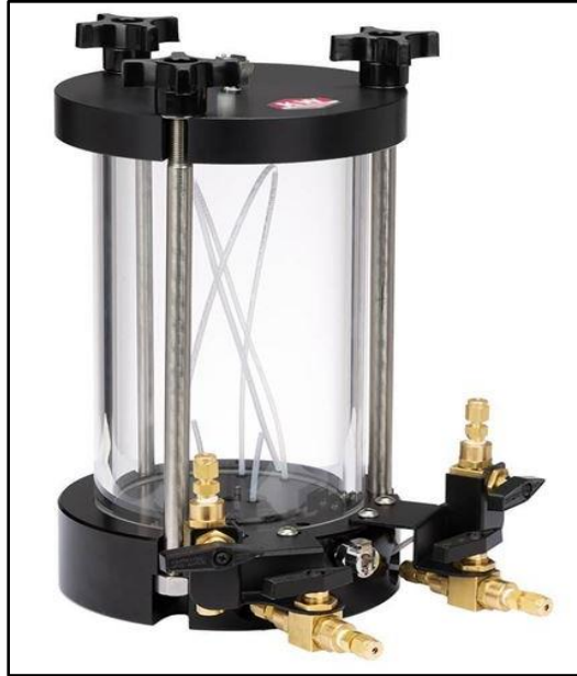
Figure A3.8: Flexible-Wall Permeability Cells for soil permeability test.
