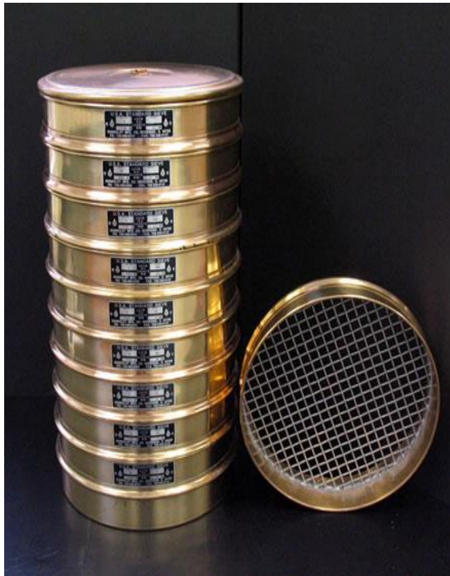
Figure A3.1: Stacked Sieves used for particle test.
