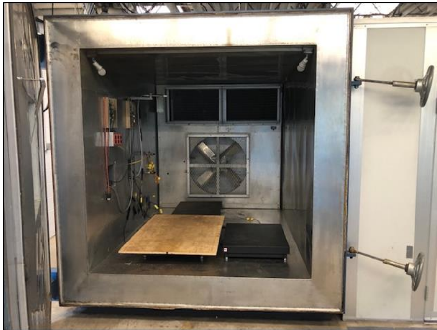
Figure 15. Environmental chamber with an inner volume of 7.79 m 3 (275 ft 3 )
