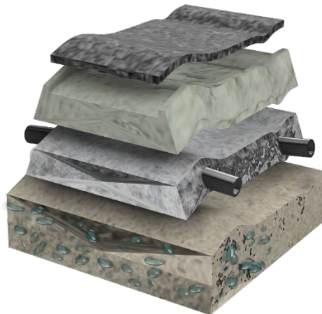
Figure 18. Isometric view of a road section with freeze/thaw damage in the vicinity of a culvert.
