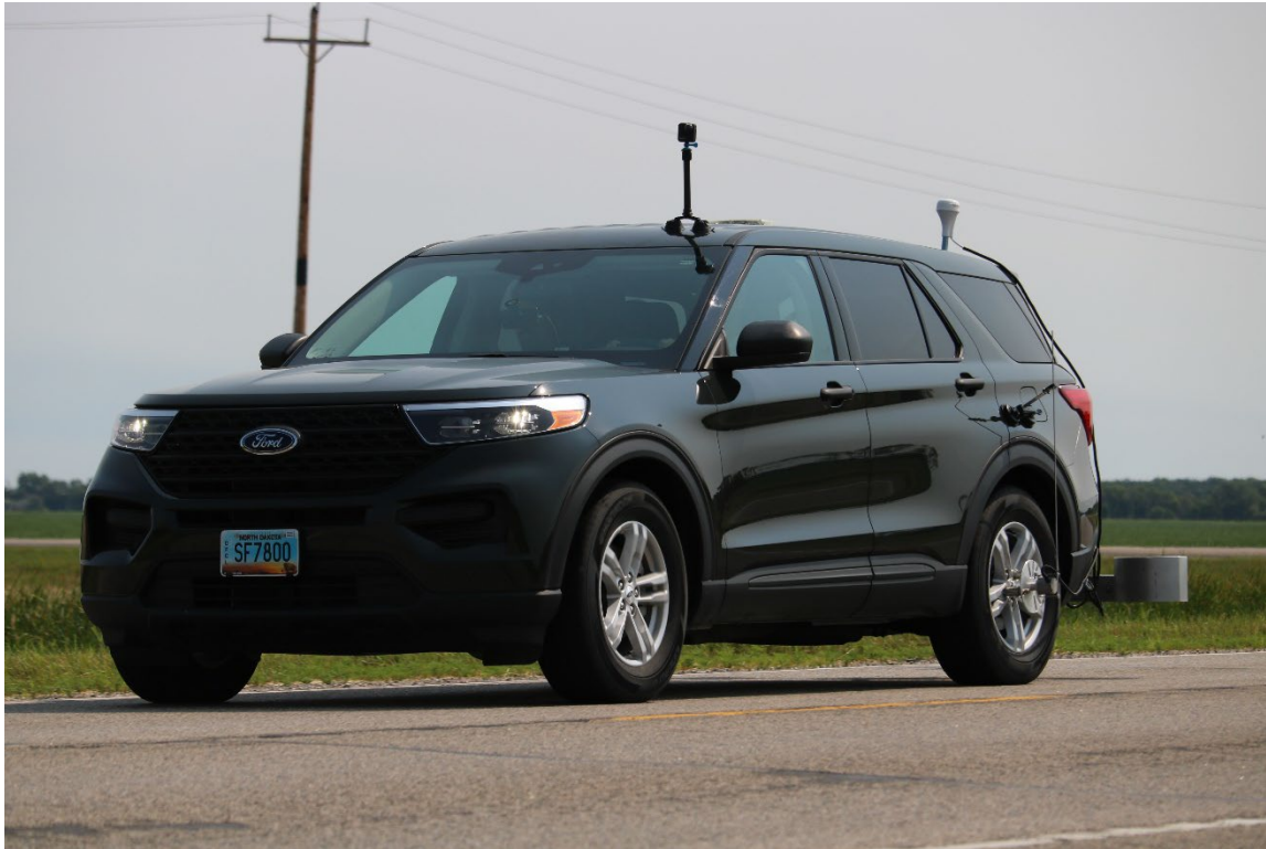
Figure H.1. UGPTI Utilized a Portable Profiler for Pavement Data Collection
