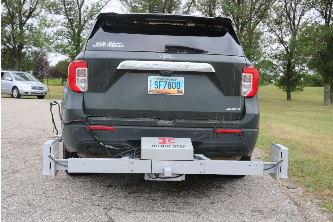
Figure H.2. IRISgo Portable Profiler for Pavement Data Collection
