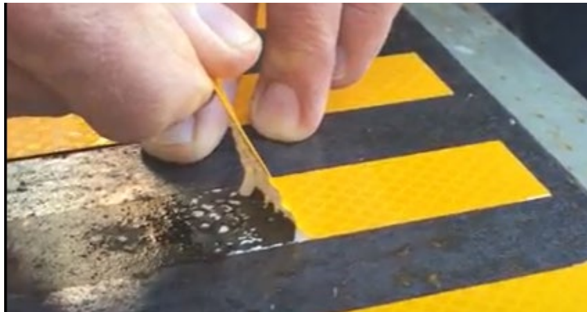
Figure 30. 3M specimen adhered to steel 6-month adhesion pull-off test.
