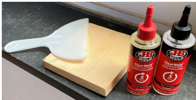
(a) Epoxy materials used to adhere sensor to concrete substrate.
