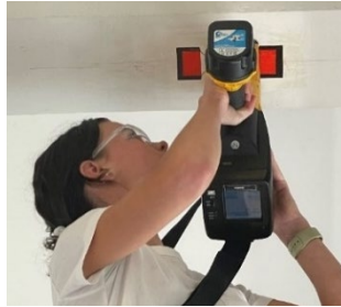
(b) Take retroreflective readings of the installed sensor.
