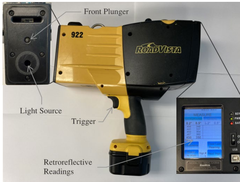
Figure 19. RoadVista 922 handheld retroreflectometer
