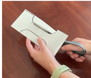
(b) Trim Excess RRSM so that the sensor is a “dog bone” shape
