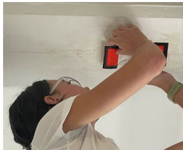
(a) Remove backing film from RRSM and apply sensor to epoxy-coated substrate.
