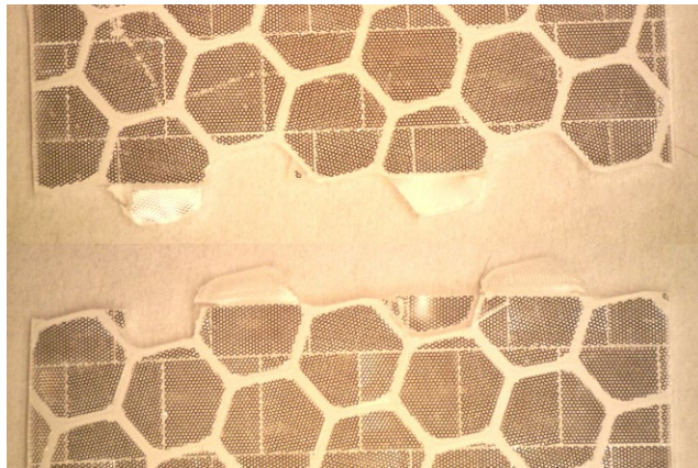
(a) ADTIV failure surface
