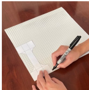
(c) Trace template onto RRSM
