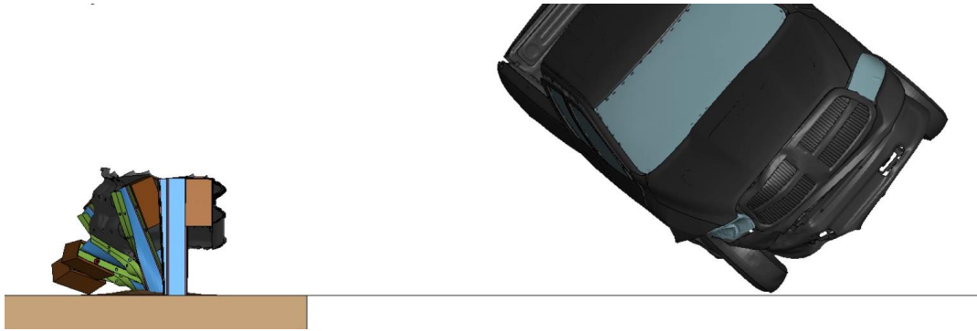
Figure 82. Maximum Roll of Pickup Truck after Exiting System (T = 0.93 sec).
