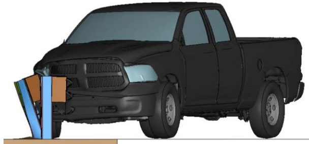
Figure 79. Front Tire of Pickup Truck Contacts Post in RTGS (T = 0.08 sec).
