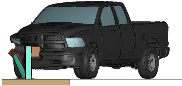
Figure 90. Front Tire of Pickup Truck Interacts with Post (T = 0.1 sec).
