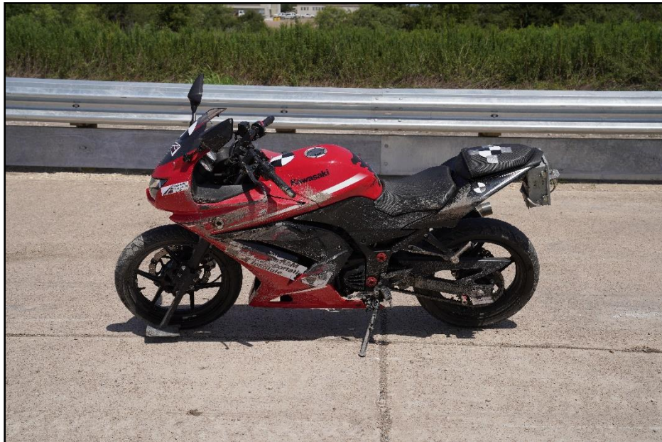
Figure 11.9. Opposite Impact Side of Test Vehicle after Test 469940-03-3.
