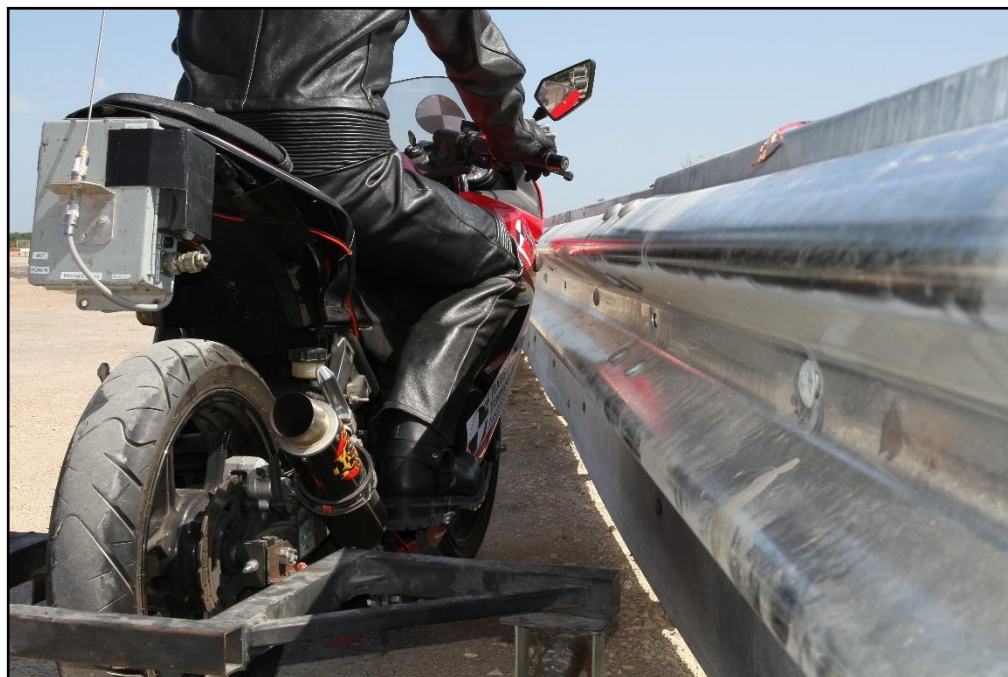
Figure 11.2. Enhanced Motorcycle Guard Fence System/Test Vehicle Impact Location for Test 469940-03-3.
