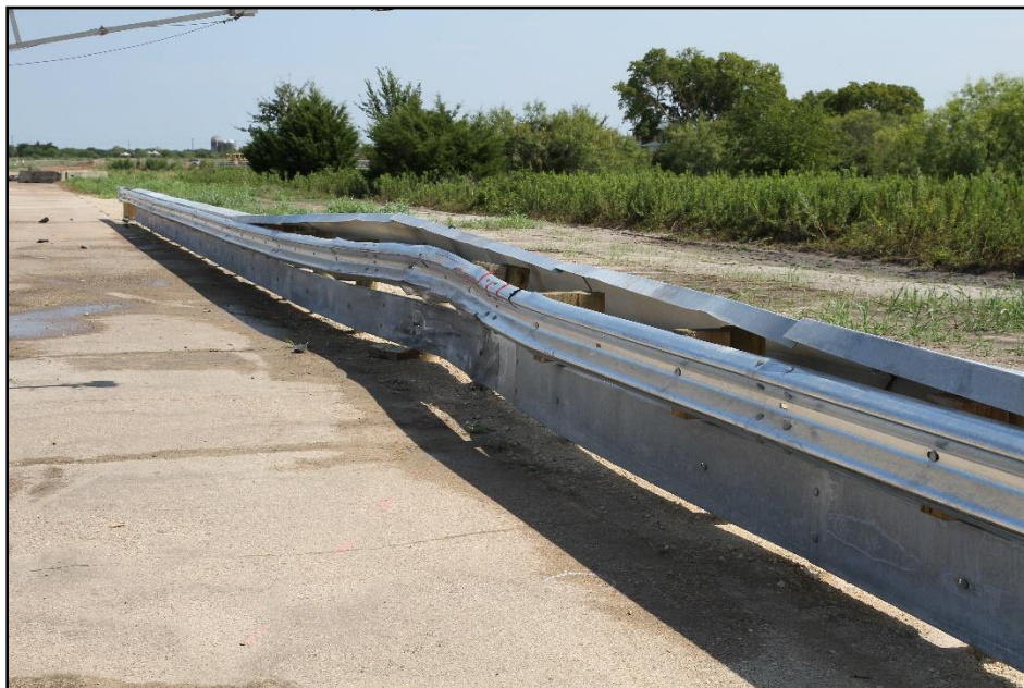
Figure 9.5. Enhanced Motorcycle Guard Fence System at Impact Location after Test 469940-03-1.
