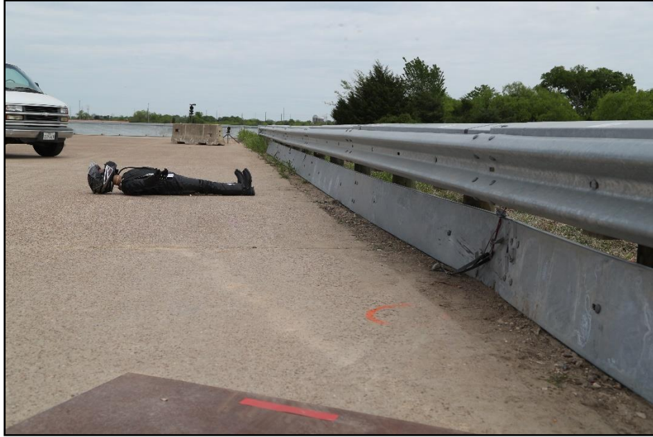
Figure 16.3. Enhanced Motorcycle Guard Fence System at Impact Location after Test 469943-01-1A.
