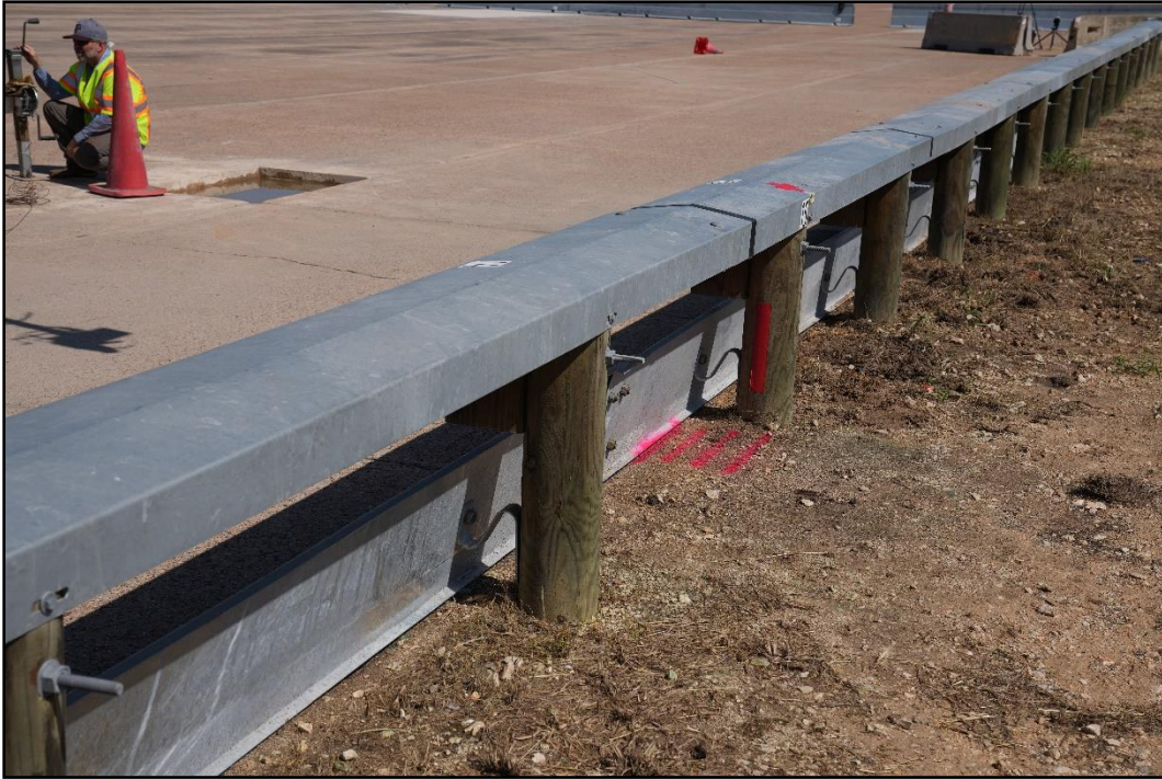
Figure 6.9. Field-Side View of the Enhanced Motorcycle Guard Fence System prior to Testing for 469942-01-1.
