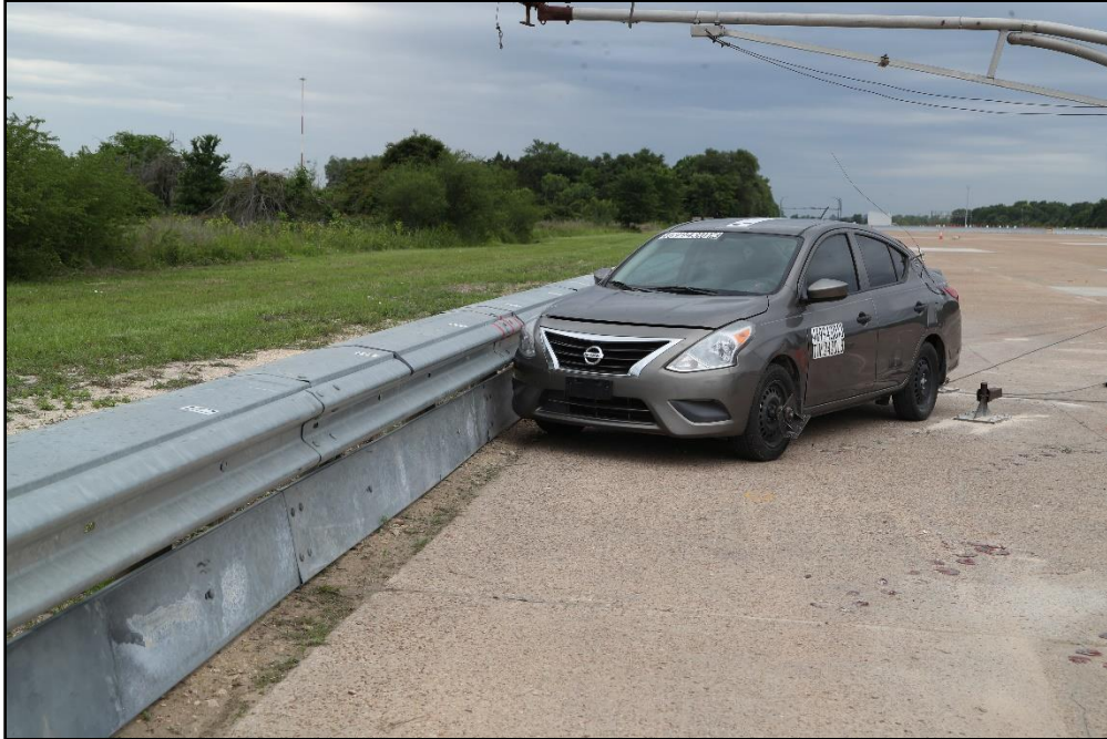
Figure 18.1. Enhanced Motorcycle Guard Fence System/Test Vehicle Geometrics for Test 469943-01-3.
