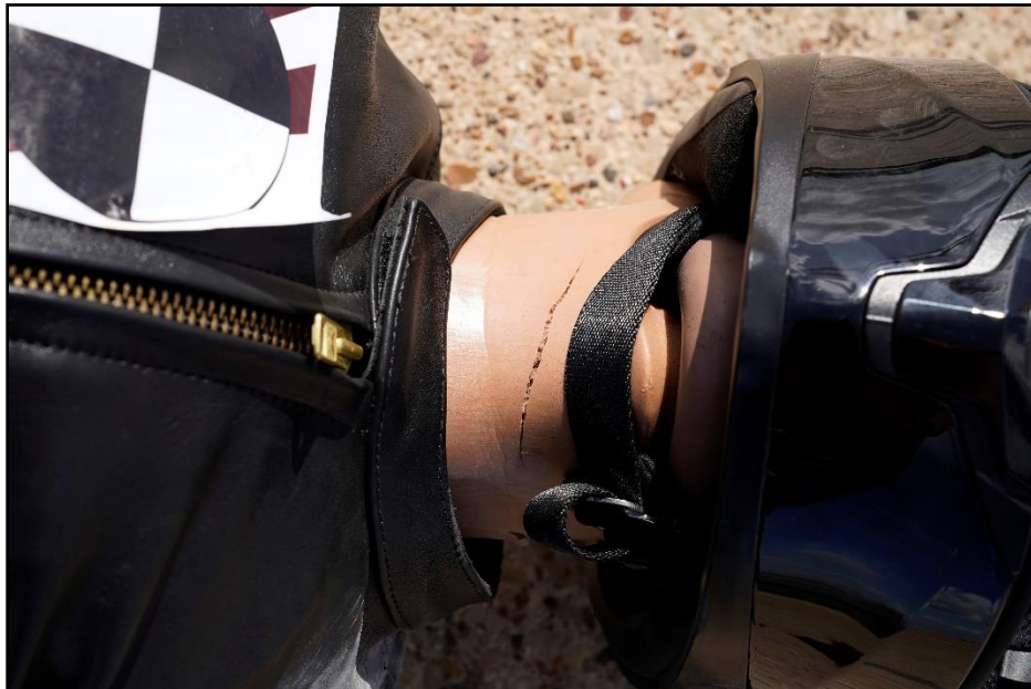
Figure 12.8. ATD Neck Damage after Test 469940-03-4A.
