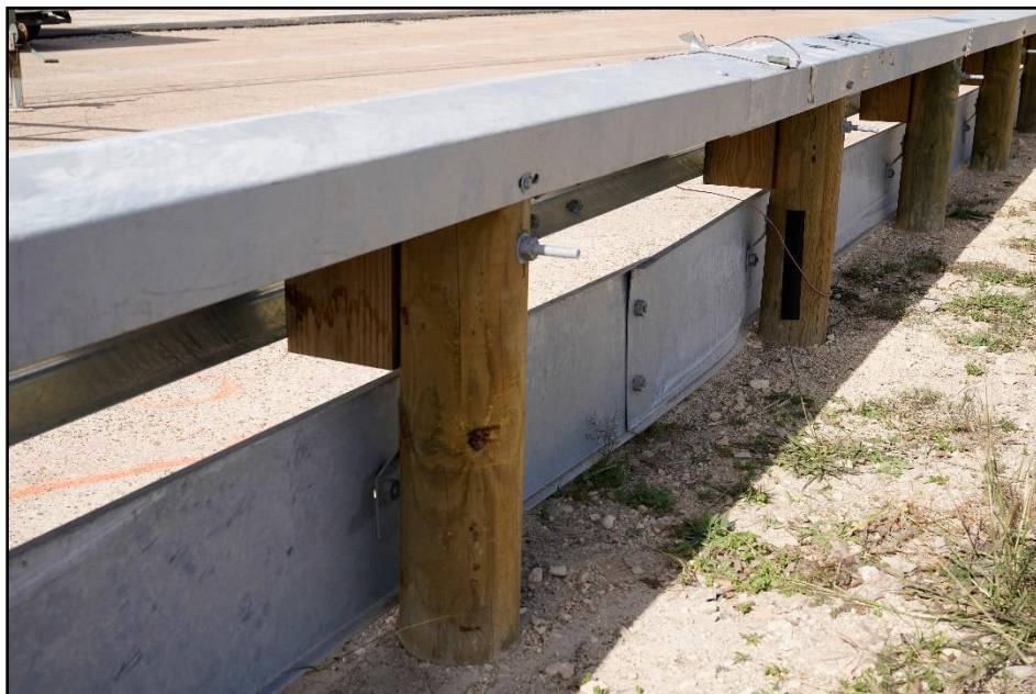
Figure 12.4. Enhanced Motorcycle Guard Fence System at Impact Location on the Field Side after Test 469940-03-4A.
