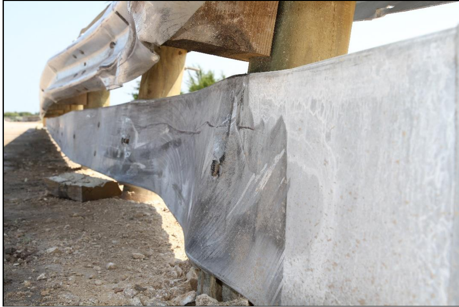
Figure 9.6. Enhanced Motorcycle Guard Fence System at the Rubrail at Impact after Test 469940-03-1.
