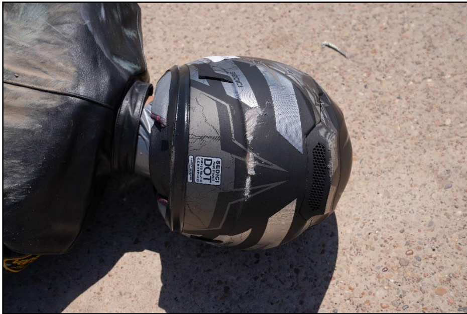
Figure 14.8. Backside Detail of the ATD Helmet after Test 469942-01-1.
