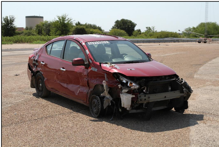
Figure 9.7. Impact Side of Test Vehicle after Test 469940-03-1.
