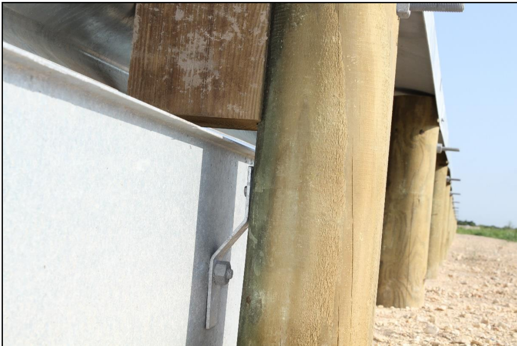
Figure 6.5. Enhanced Motorcycle Guard Fence System Rubrail Bracket Detail prior to Testing for 469940-03-1, 469940-03-2, 469940-03-3, and 469940-03-4A.
