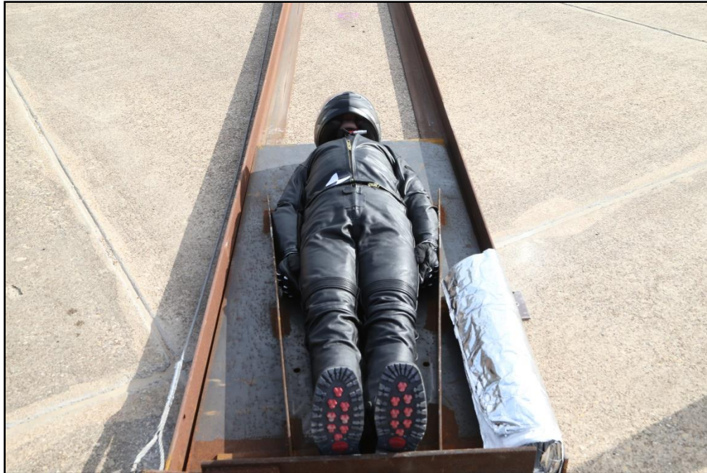
Figure 17.2. In-Line View of the ATD on the Sled Delivery System prior to Test 469943-01-2.
