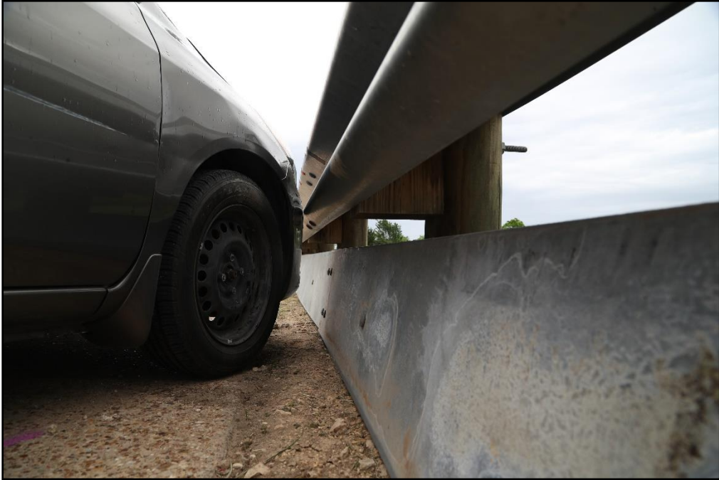
Figure 18.2. Enhanced Motorcycle Guard Fence System/Test Vehicle Impact Location for Test 469943-01-3.
