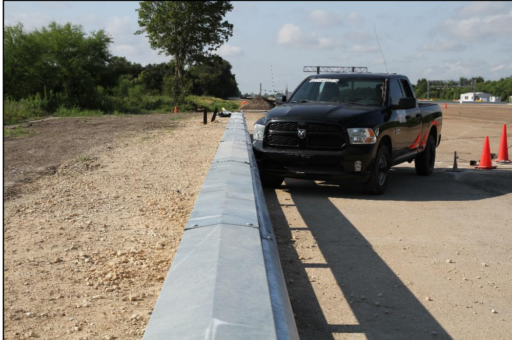
Figure 10.1. Enhanced Motorcycle Guard Fence System/Test Vehicle Geometrics for Test 469940-03-2.
