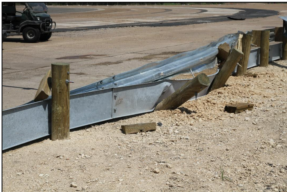
Figure 10.6. Enhanced Motorcycle Guard Fence System at Impact Location on the Field Side after Test 469940-03-2.
