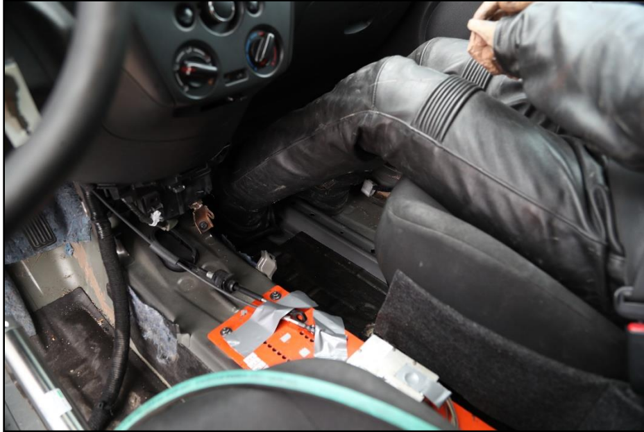
Figure 18.10. Interior of Test Vehicle on Impact Side after Test 469943-01-3.
