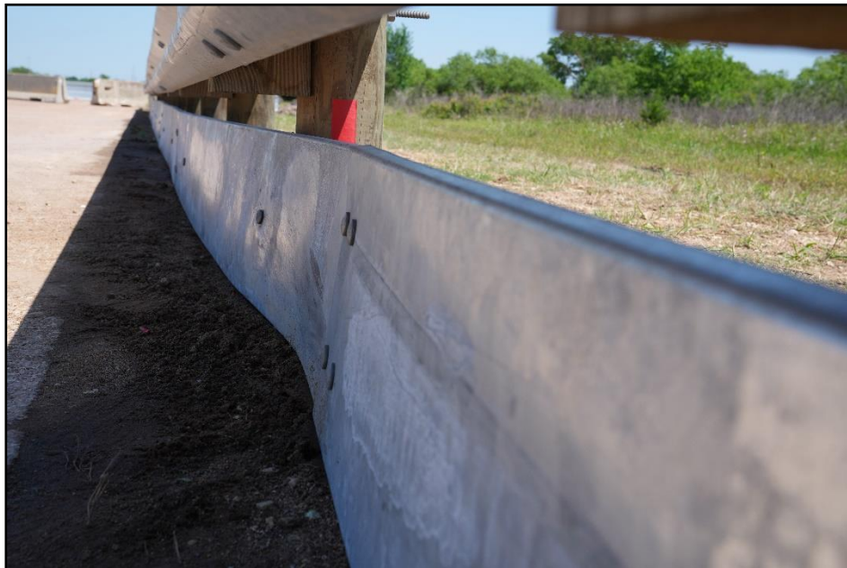
Figure 14.4. Enhanced Motorcycle Guard Fence System Rubrail at Impact Location after Test 469942-01-1.
