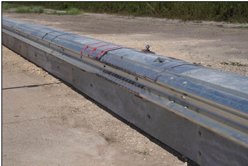
Figure 11.5. Isometric View of the Enhanced Motorcycle Guard Fence System at Impact Location after Test 469940-03-3.
