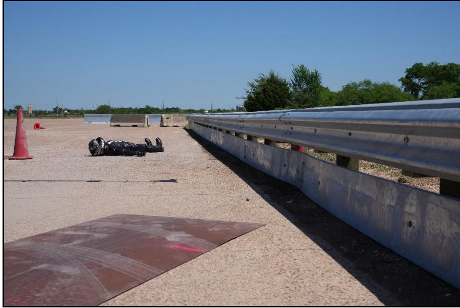
Figure 14.3. Enhanced Motorcycle Guard Fence System at Impact Location after Test 469942-01-1.
