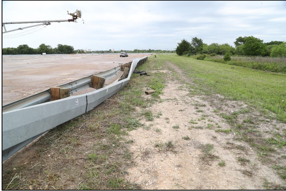
Figure 18.6. Field-Side View of the Enhanced Motorcycle Guard Fence System at Impact Location after Test 469943-01-3.
