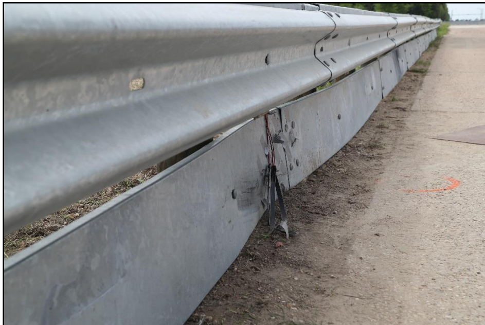
Figure 16.4. Enhanced Motorcycle Guard Fence System Rubrail at Impact Location after Test 469943-01-1A.
