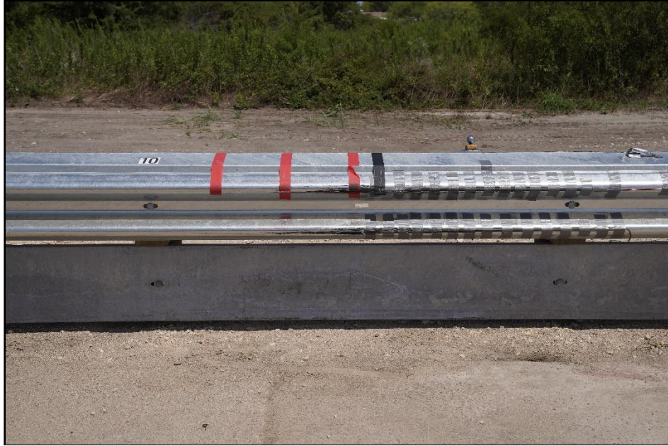
Figure 11.6. Elevation View of the Enhanced Motorcycle Guard Fence System at Impact Location after Test 469940-03-3.
