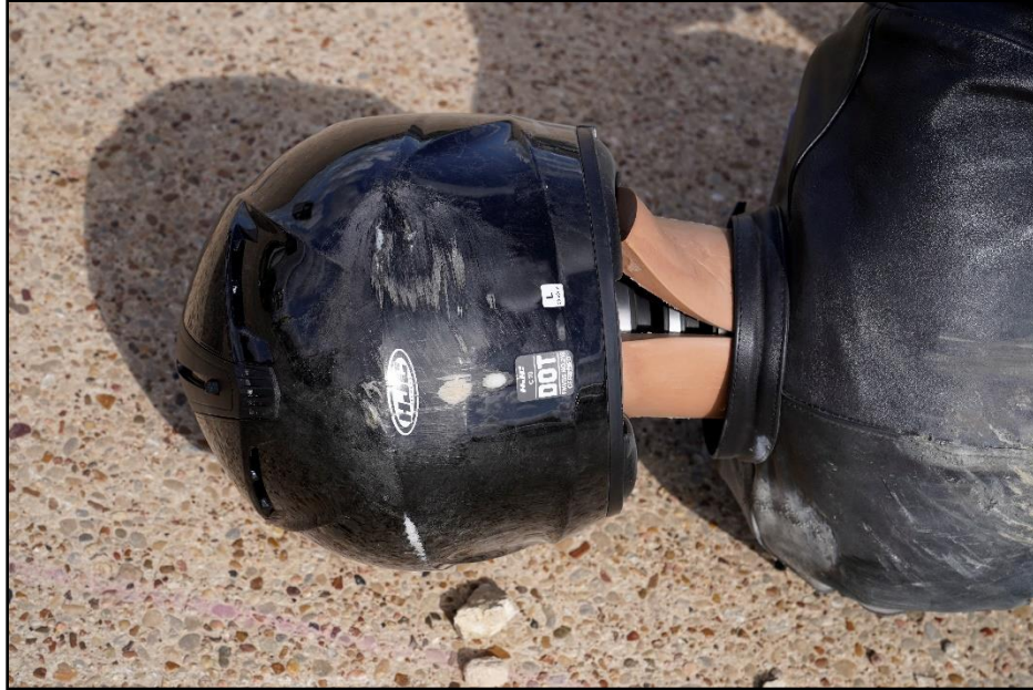
Figure 12.7. Back Helmet and ATD Neck Damage after Test 469940-03-4A.
