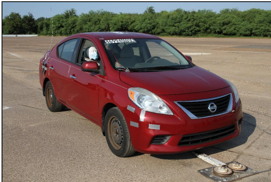
Figure 9.3. Impact Side of Test Vehicle before Test 469940-03-1.
