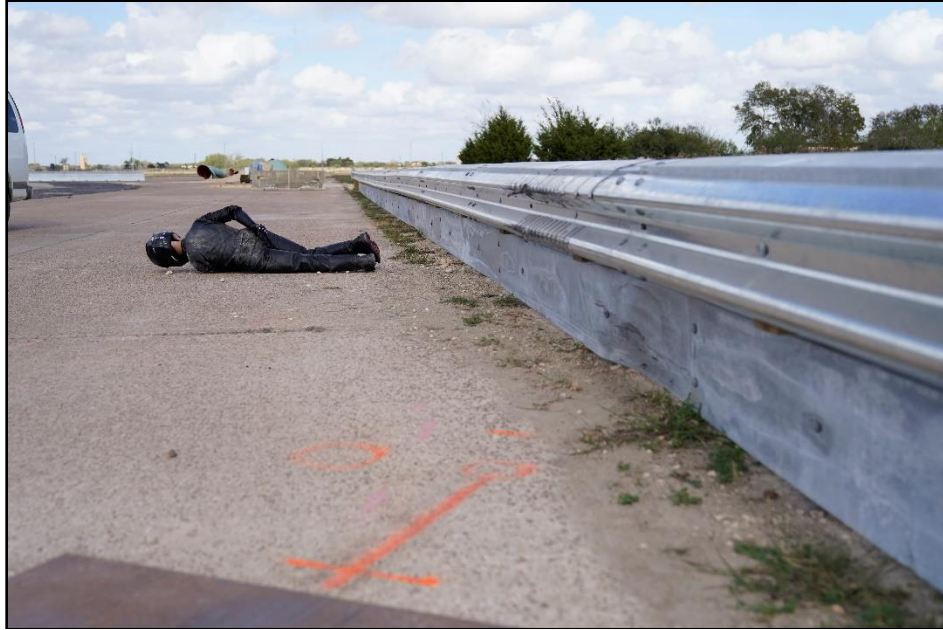
Figure 12.3. Enhanced Motorcycle Guard Fence System at Impact Location on the Traffic Side after Test 469940-03-4A.
