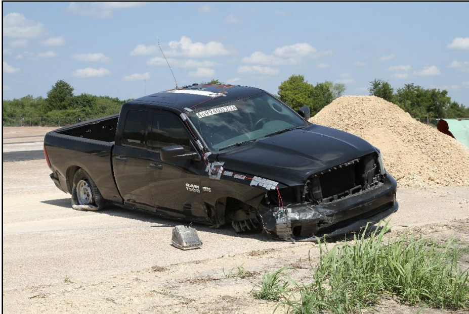
Figure 10.7. Impact Side of Test Vehicle after Test 469940-03-2.
