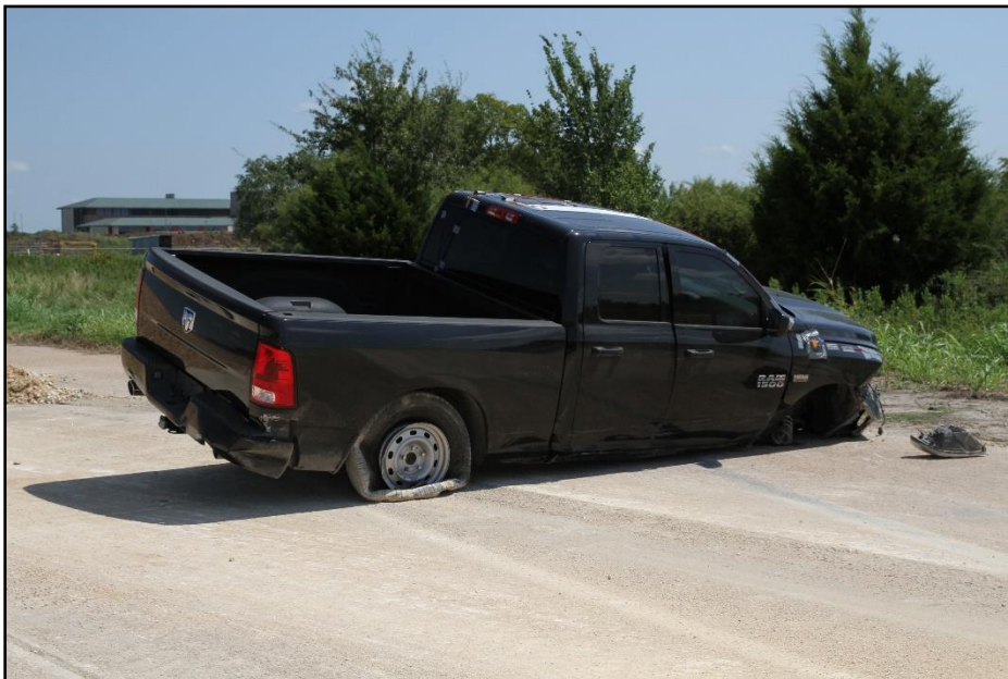
Figure 10.8. Rear Impact Side of Test Vehicle after Test 469940-03-2.
