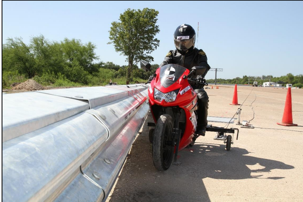
Figure 11.1. Enhanced Motorcycle Guard Fence System/Test Vehicle Geometrics for Test 469940-03-3.
