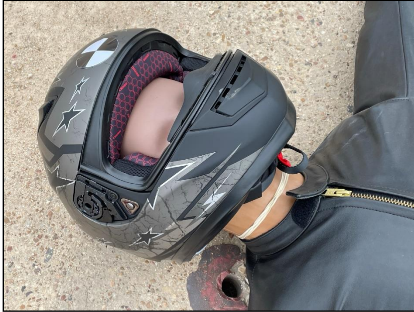
Figure 17.7. Helmet Damage after Test 469943-01-2.
