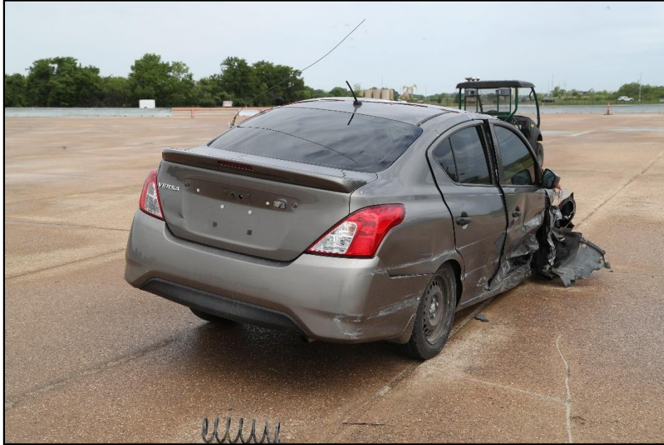
Figure 18.8. Rear Impact Side of Test Vehicle after Test 469943-01-3.
