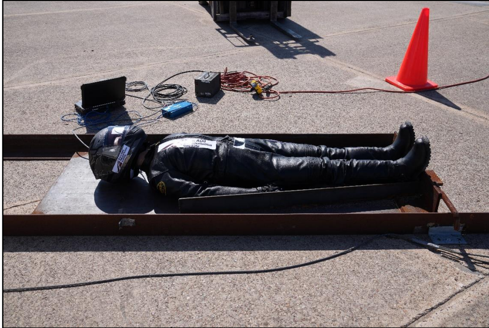
Figure 14.1. Side View of the ATD on the Sled Delivery System Prior to Test 469942-01-1.
