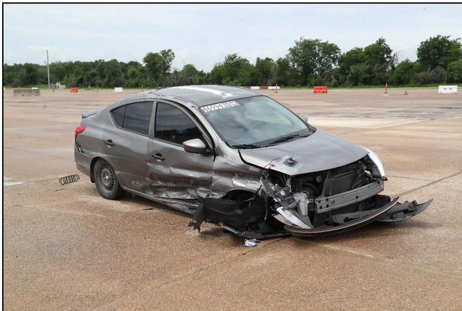
Figure 18.7. Impact Side of Test Vehicle after Test 469943-01-3.
