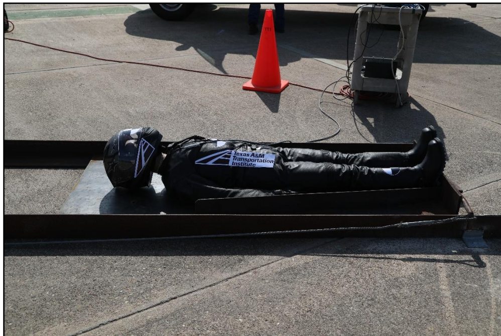
Figure 16.1. Side View of the ATD on the Sled Delivery System prior to Test 469943-01-1A.
