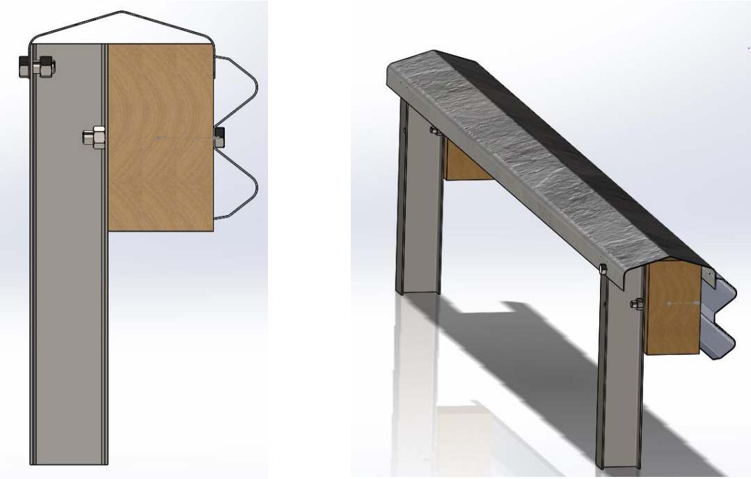
Figure 4.1. Option 1 Conceptual Drawing for Bent Plate Top Protection.
