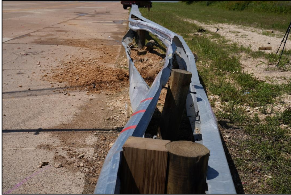
Figure 19.6. In-Line View of the Enhanced Motorcycle Guard Fence System at Impact Location after Test 469943-01-4.
