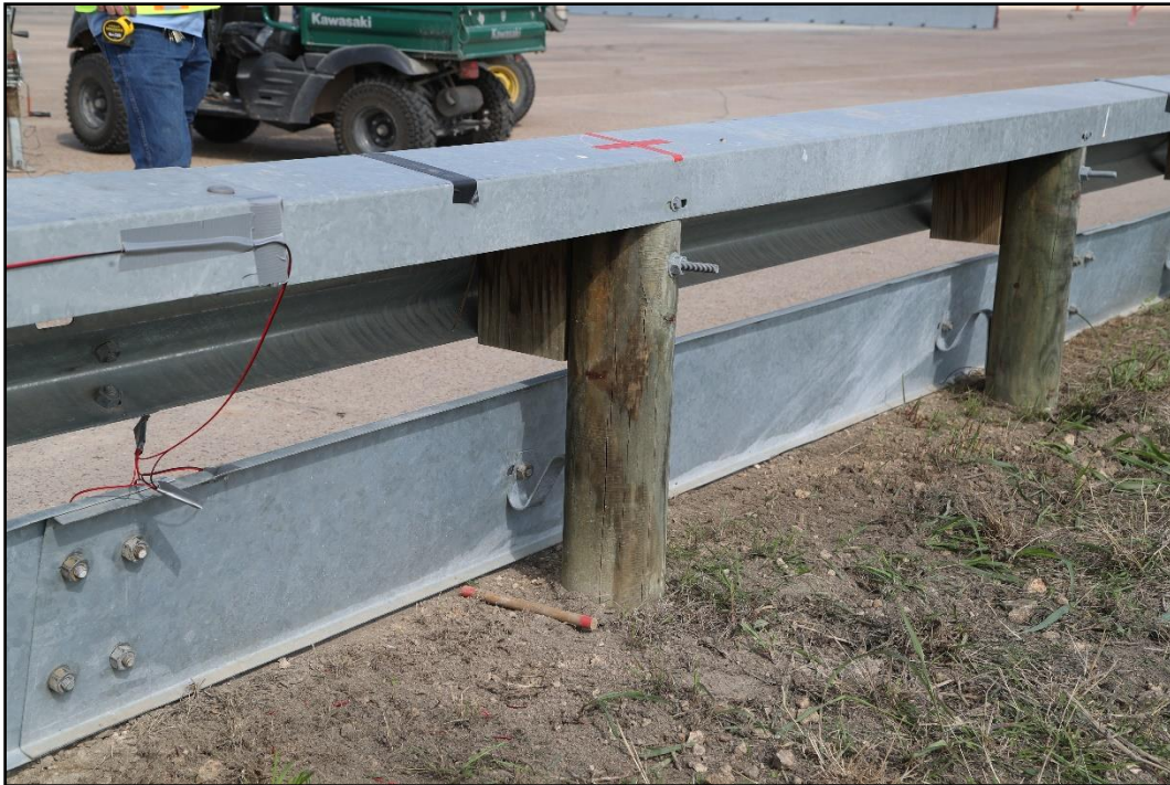
Figure 6.12. Field-Side View of the Enhanced Motorcycle Guard Fence System prior to Testing for 469943-01-1A, 469943-01-2, 469943-01-3, and 469943-01-4.
