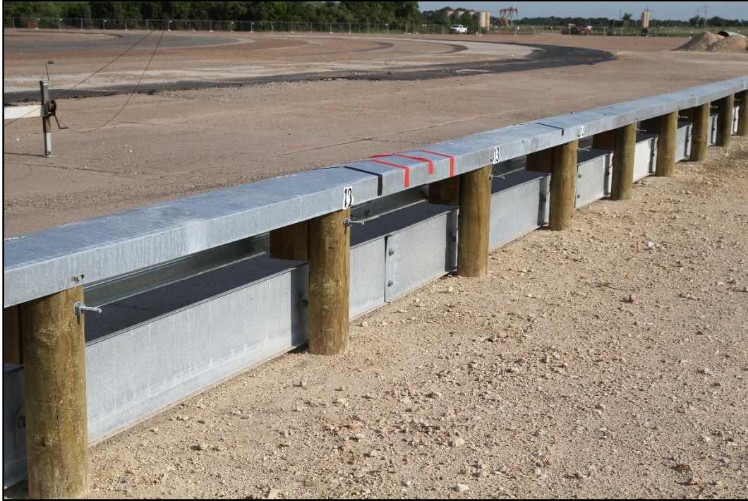
Figure 6.4. Field-Side View of the Enhanced Motorcycle Guard Fence System prior to Testing for 469940-03-1, 469940-03-2, 469940-03-3, and 469940-03-4A.
