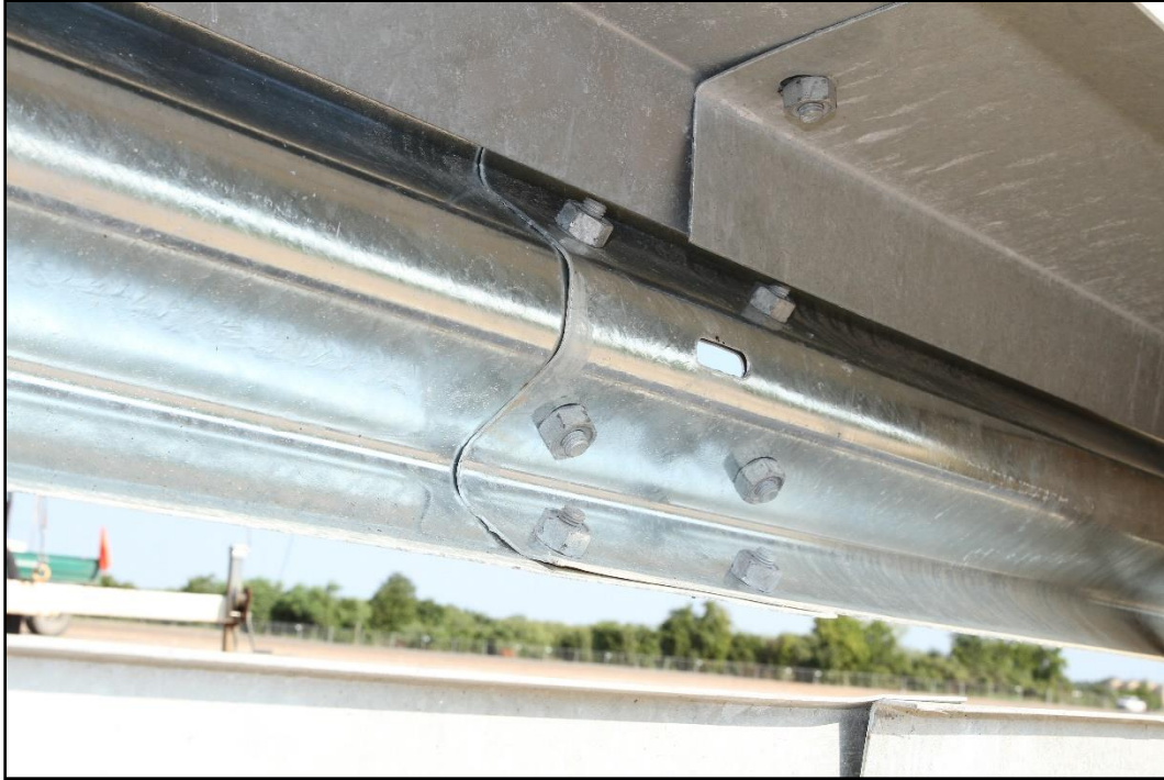
Figure 6.6. Enhanced Motorcycle Guard Fence System W-Beam Hardware Detail prior to Testing for 469940-03-1, 469940-03-2, 469940-03-3, and 469940-03-4A.
