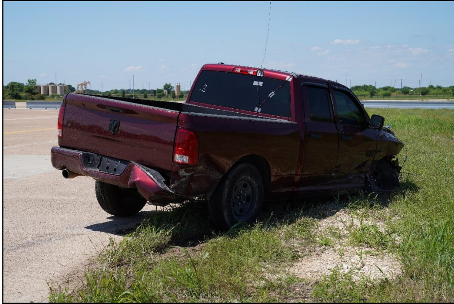
Figure 19.8. Rear Impact Side of Test Vehicle after Test 469943-01-4.
