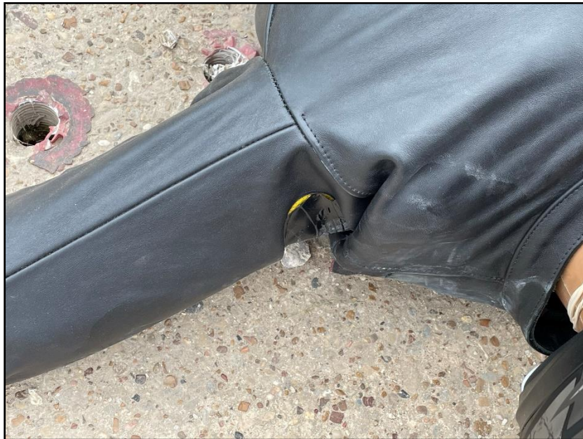
Figure 17.8. Shoulder Damage after Test 469943-01-2.
