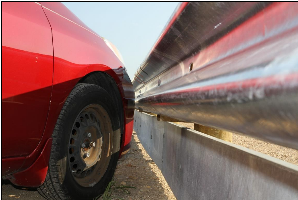
Figure 9.2. Enhanced Motorcycle Guard Fence System/Test Vehicle Impact Location for Test 469940-03-1.
