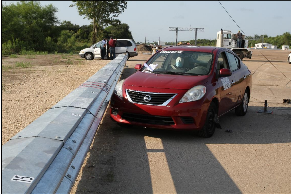
Figure 9.1. Enhanced Motorcycle Guard Fence System/Test Vehicle Geometrics for Test 469940-03-1.
