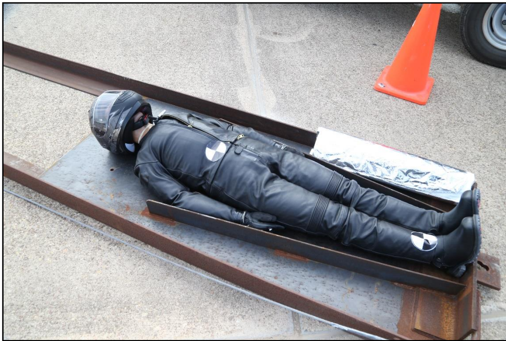
Figure 17.1. Side View of the ATD on the Sled Delivery System prior to Test 469943-01-2.
