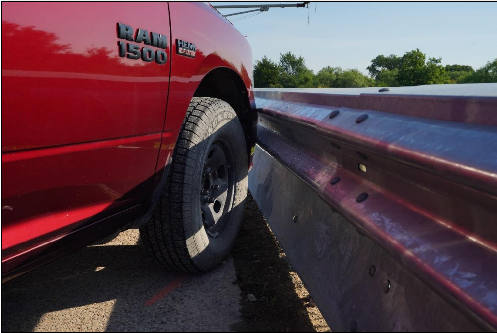
Figure 19.2. Enhanced Motorcycle Guard Fence System/Test Vehicle Impact Location for Test 469943-01-4.
