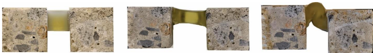
Figure 62: Residual deformation after applying 100% at 3 mm/h displacement rate
