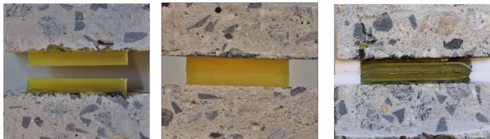
Figure 25. Illustration of applying controlled displacement for self-healing of sealants in concrete joints under ambient conditions
