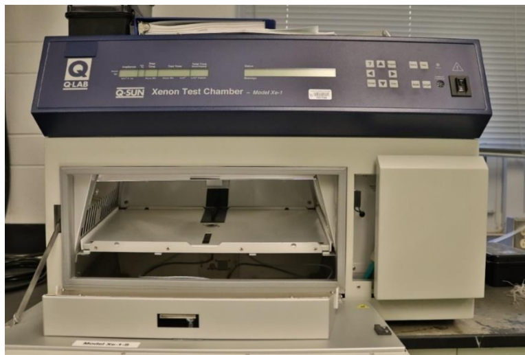
Figure 23. Q-SUN Xe-1 xenon test chamber
