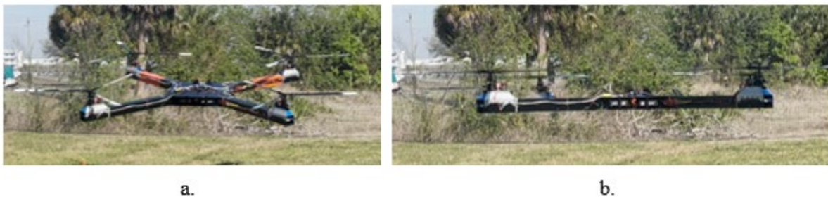
Figure 97. a) Vehicle tracking pilot pitch command. b) Vehicle returning to level when no pilot input commanded
