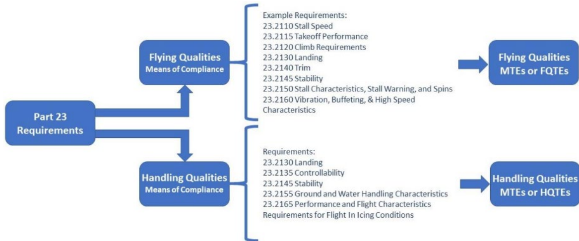
Figure 14. Mission task elements as a means of compliance
