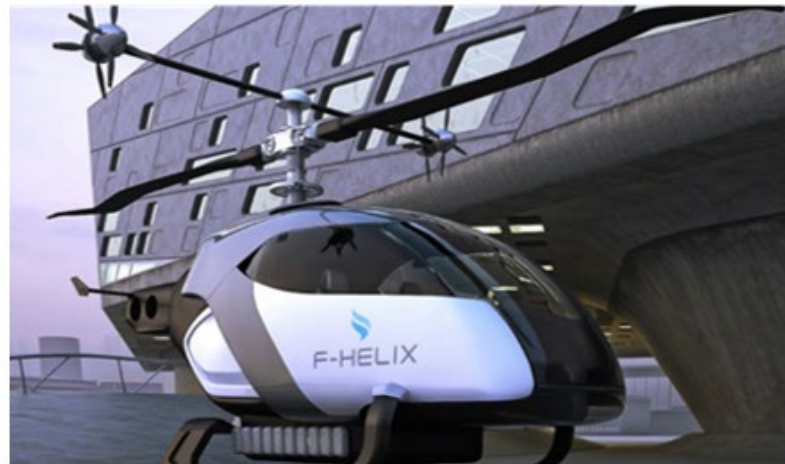
Figure 1. Artistic renditions of the Jaunt Air Mobility slowed rotor compound helicopter (a) and the Vinati F-Helix propeller reaction-driven helicopter eVTOL (b) concepts (images from https://evtol.news )
