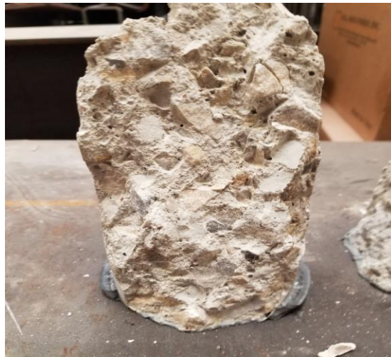
Figure 4.19: Typical compression failure through cementitious paste
