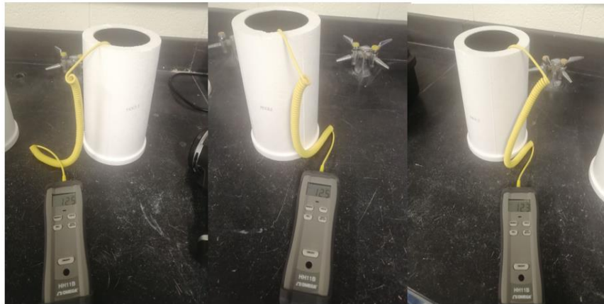
Figure 4.1: Water temperature readings in each cylinder showing mold 1, 2 and 3 from left to right
