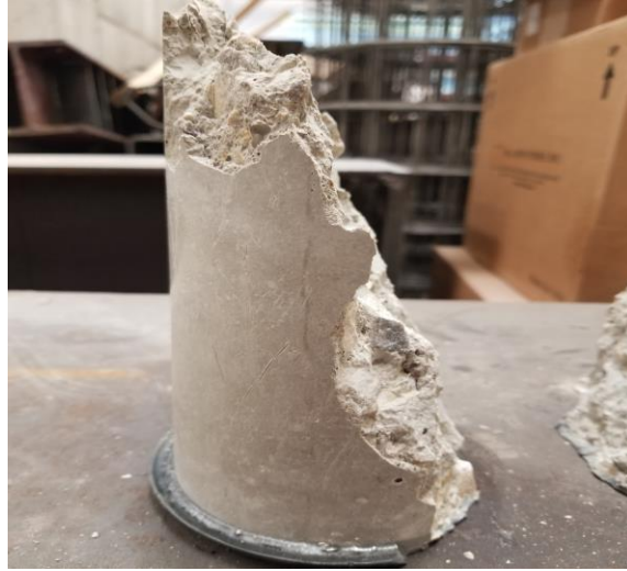
Figure 4.18: Typical type I compression failure plane
