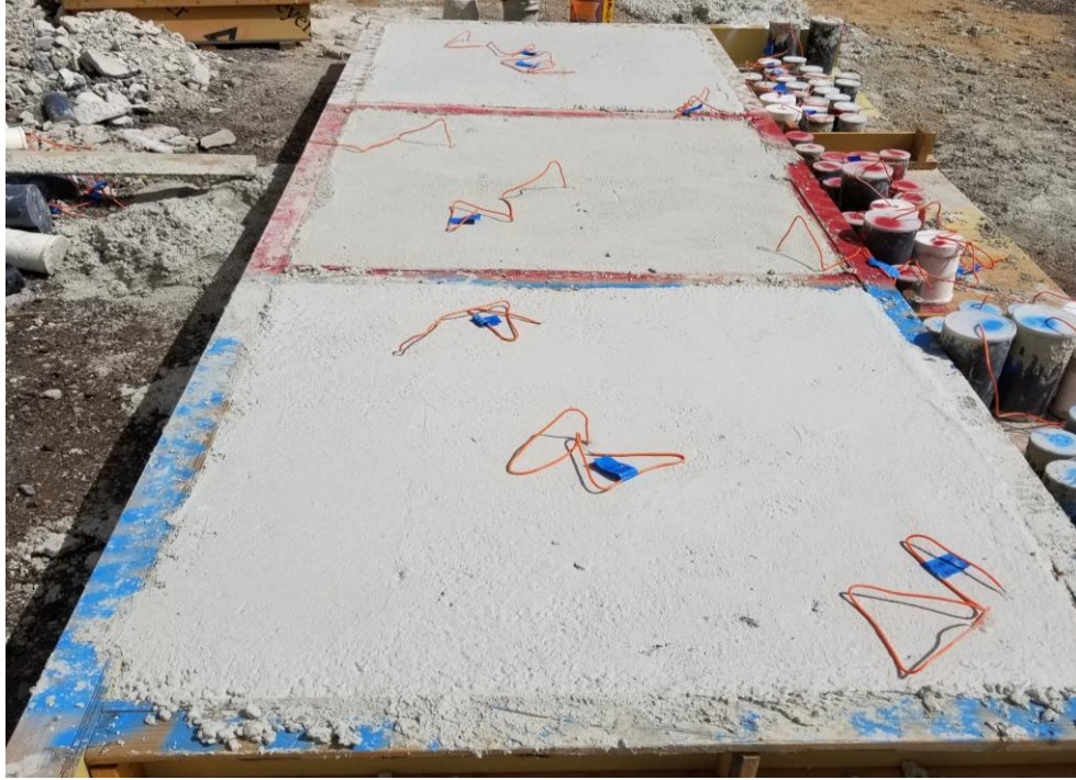
Figure 4.15: Color labeling on 5'x5'x9" large in-situ slabs
