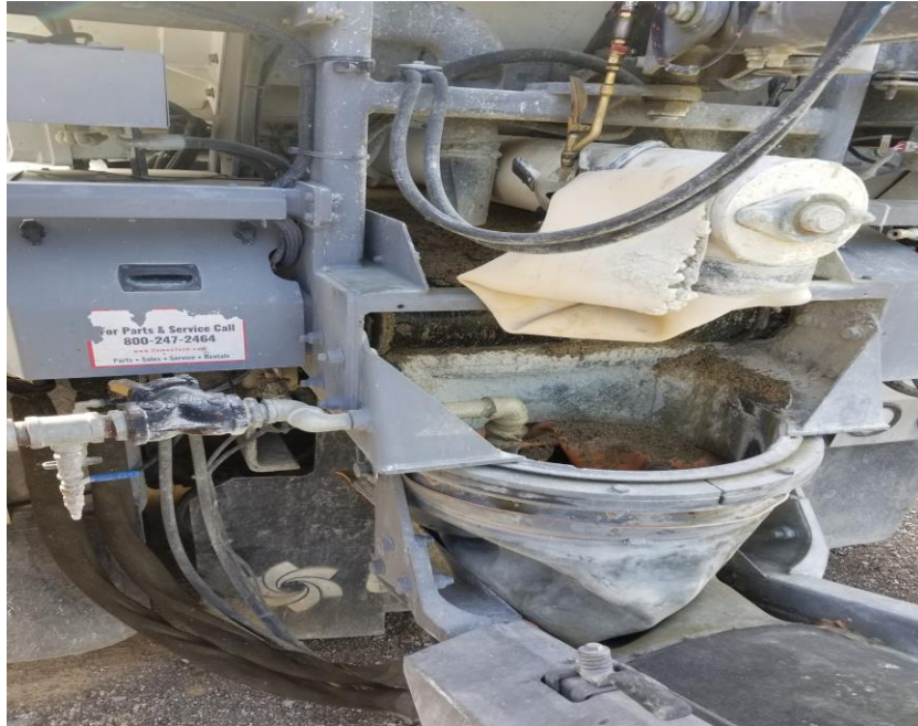
Figure 4.7: Hopper at the mixing auger
