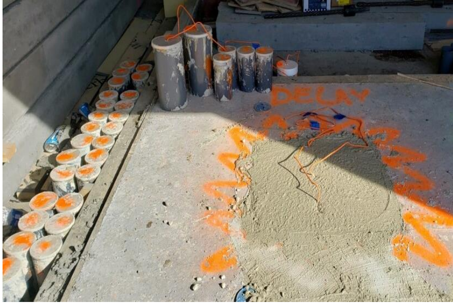
Figure 4.10: Curing of cast specimens
