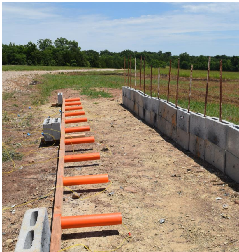
Figure 5. Impact Sensitivity Test Setup. Mortar tubes were lined up facing a cinderblock wall (3 feet away). Commercial and custom pyrotechnic products were loaded and ignited, resulting in each product striking the wall.
