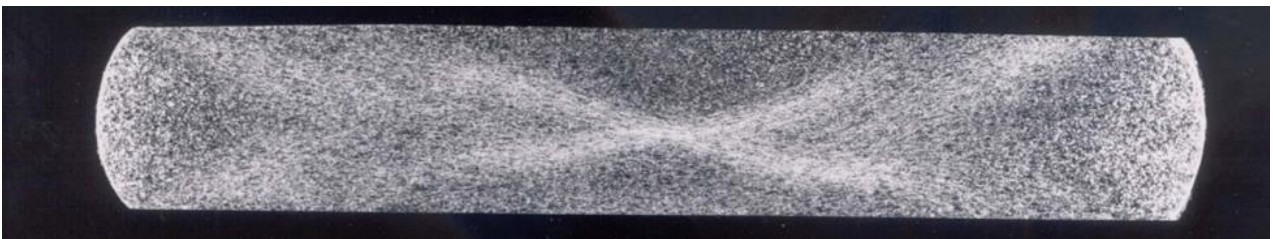
Figure 80. Extreme example of flow localization and shear band formation in Ti-6242 hot-worked at 850 °C (1562 °F)
