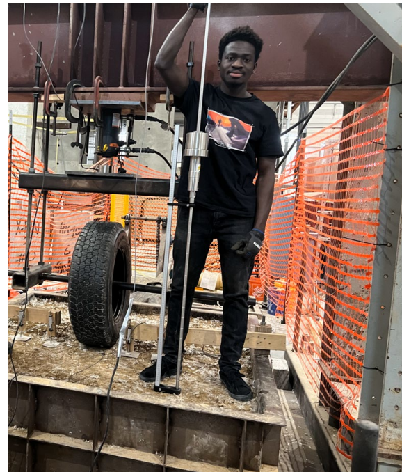
Figure 3.31 DCP test on compacted clay layer
