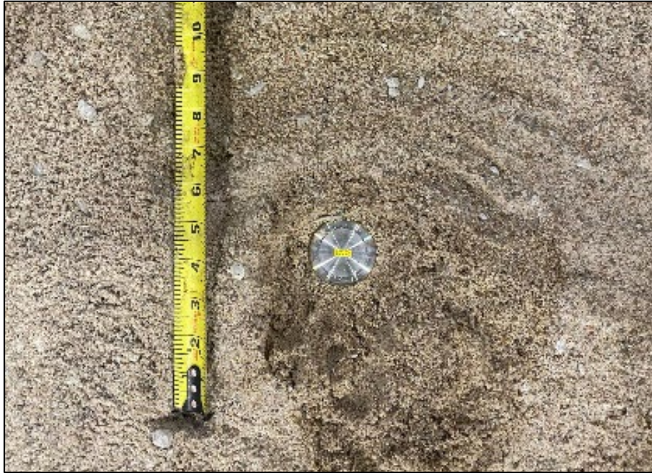
Figure 3.24 Pressure cell on compacted sand layer.
