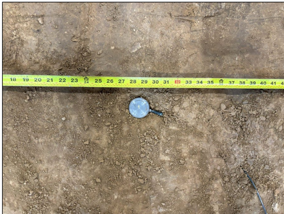
Figure 3.25 Pressure cell on compacted clay layer.
