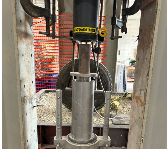
Figure 3.12 Static loading setup for UCS sample preparation
