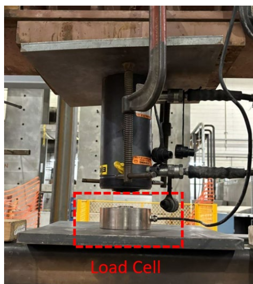
Figure 3.28 Load cell positioned beneath actuator.
