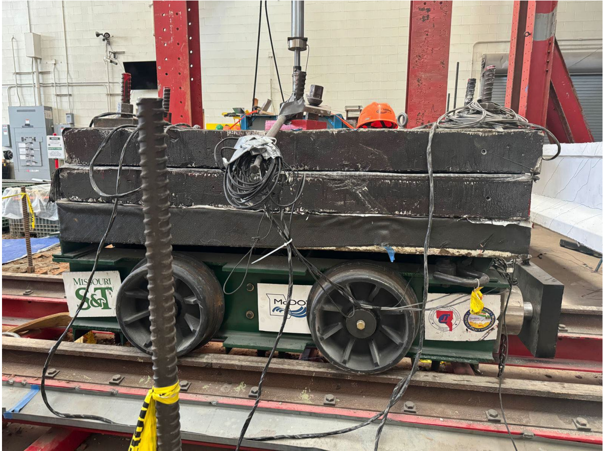
Figure 3.14 Instrumented sledge ready for impact test
