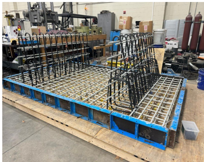
Figure 3.4 GFRP reinforcement (barrier)
