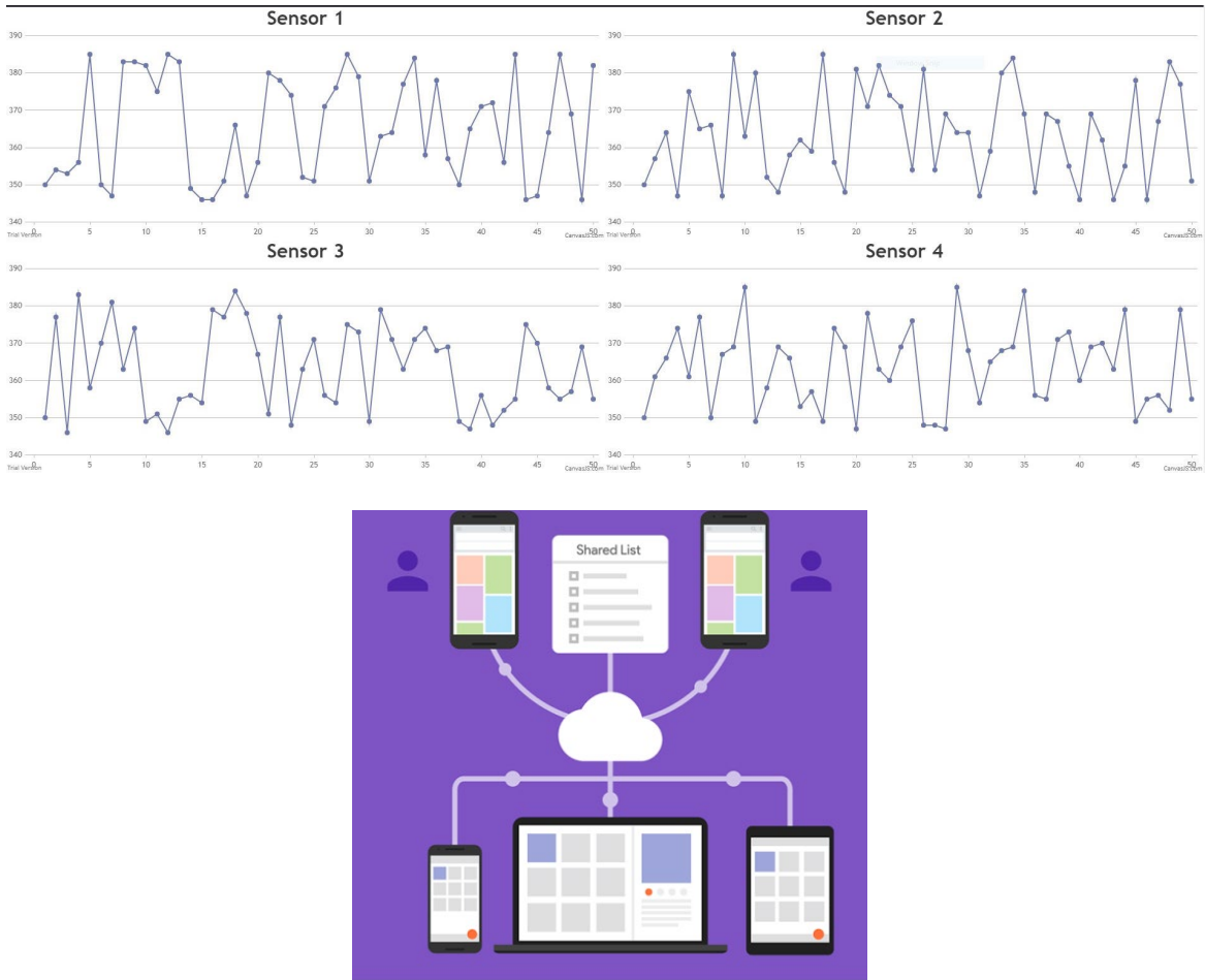
Figure 2.10 (Top panel) Sensing data uploaded to server and displayed on web app in real-time: x-axis is time in hour, y-axis is the resistance readings in ohm; (bottom panel) cloud data service by firebase.
