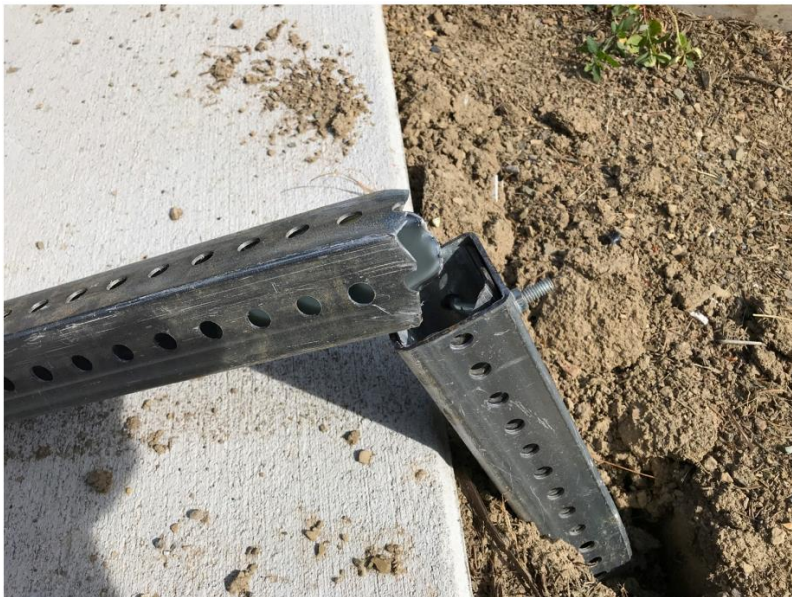
Figure E.14: The square tube breakaway post being damaged upon impact. Image courtesy of PennDOT [19].
