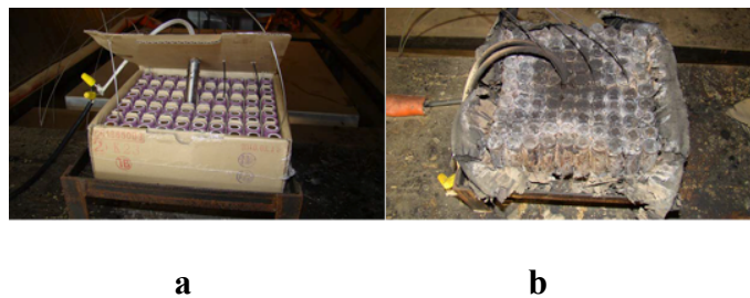
Figure 21. Shipping box with interlocking cardboard separators for 100 18650 LiCoO 2 lithium-ion cells pre and post fire [4]
