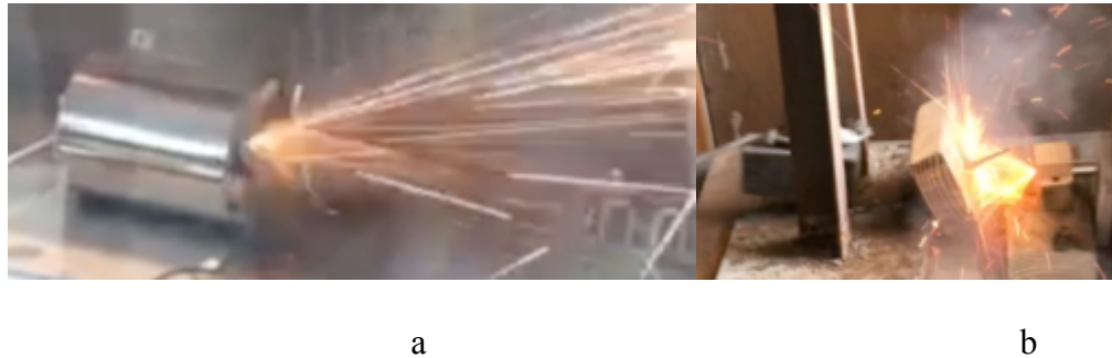
Figure 11. Li-ion battery in runaway due to a. heating in a canister, and b. abused by a sudden puncture of the battery in causing auto-ignition of the gases.
