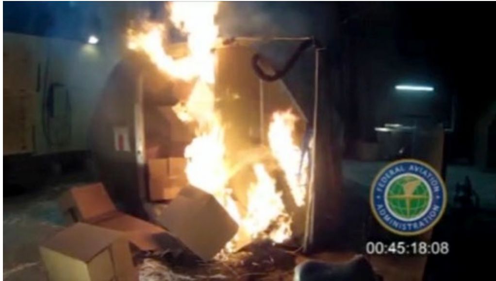
Figure 34. Cargo container explosion caused by lithium battery vent gases [30]
