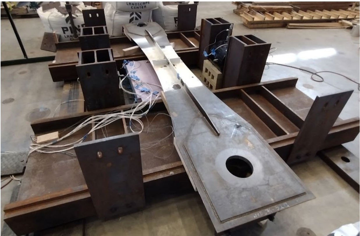
Figure 4.2 CIF specimen in place with partial self-reacting load frame
