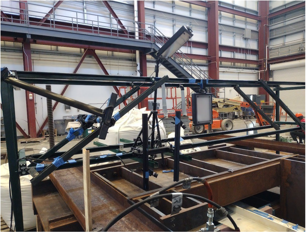
Figure 4.5 DIC cameras and lighting suspended above the CIF specimen
