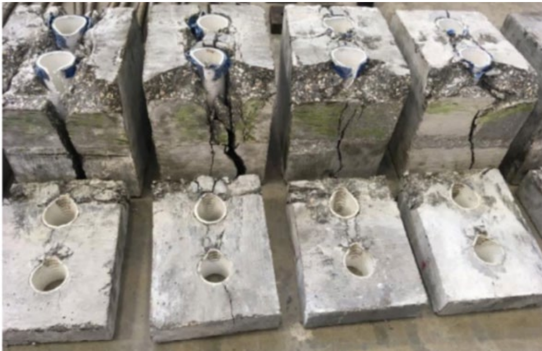
Figure 1.9 Failure mode of friction failure mode (Yuan et al. ,2018)
