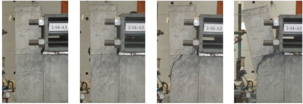
(a) Initial cracking (at the displacement of 1mm) (b) Cracks propagating (at the displacement of 5mm) (c) Cracks widening (at the displacement of 25mm) (d) End of test (at the displacement of 175mm)
