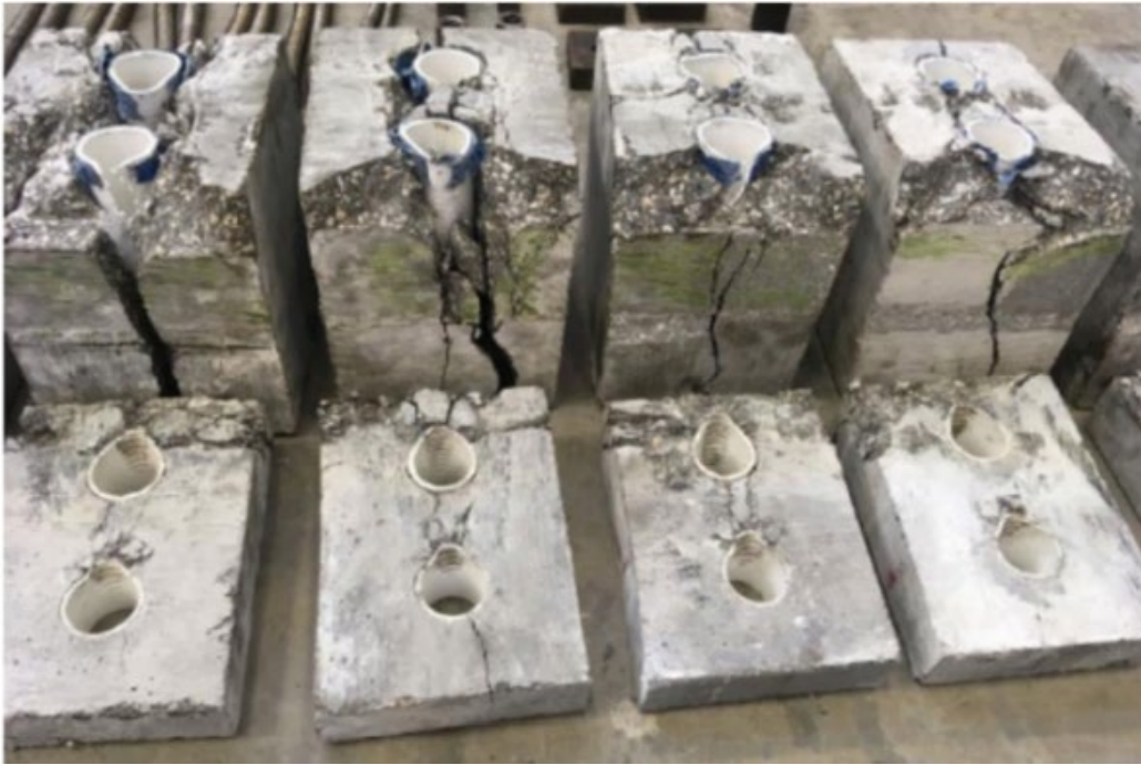
Figure 1.9 Failure mode of friction failure mode (Yuan and Chen, 2018)
