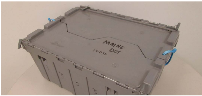
Figure 5. Tamper-resistant security tags on asphalt pavement core sample cases used by Maine DOT. Source: Maine DOT
