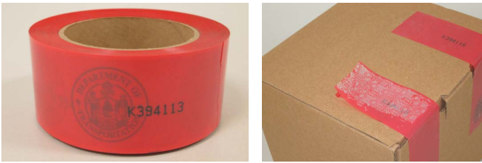
Figure 4. Security tape used by Maine DOT for asphalt mix samples. Source: Maine DOT
