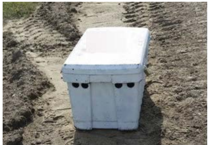
Figure 8. Use of beverage cooler for curing concrete cylinder specimen. A thermometer is placed in the curing container which is locked and clearly marked. Source: Michigan Concrete Association.
