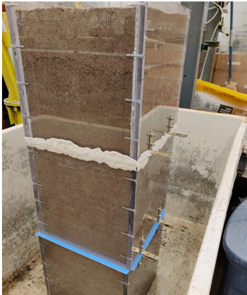
Figure 3.8 Field moisture capacity test on a 900-mm high soil column with clean sand.
