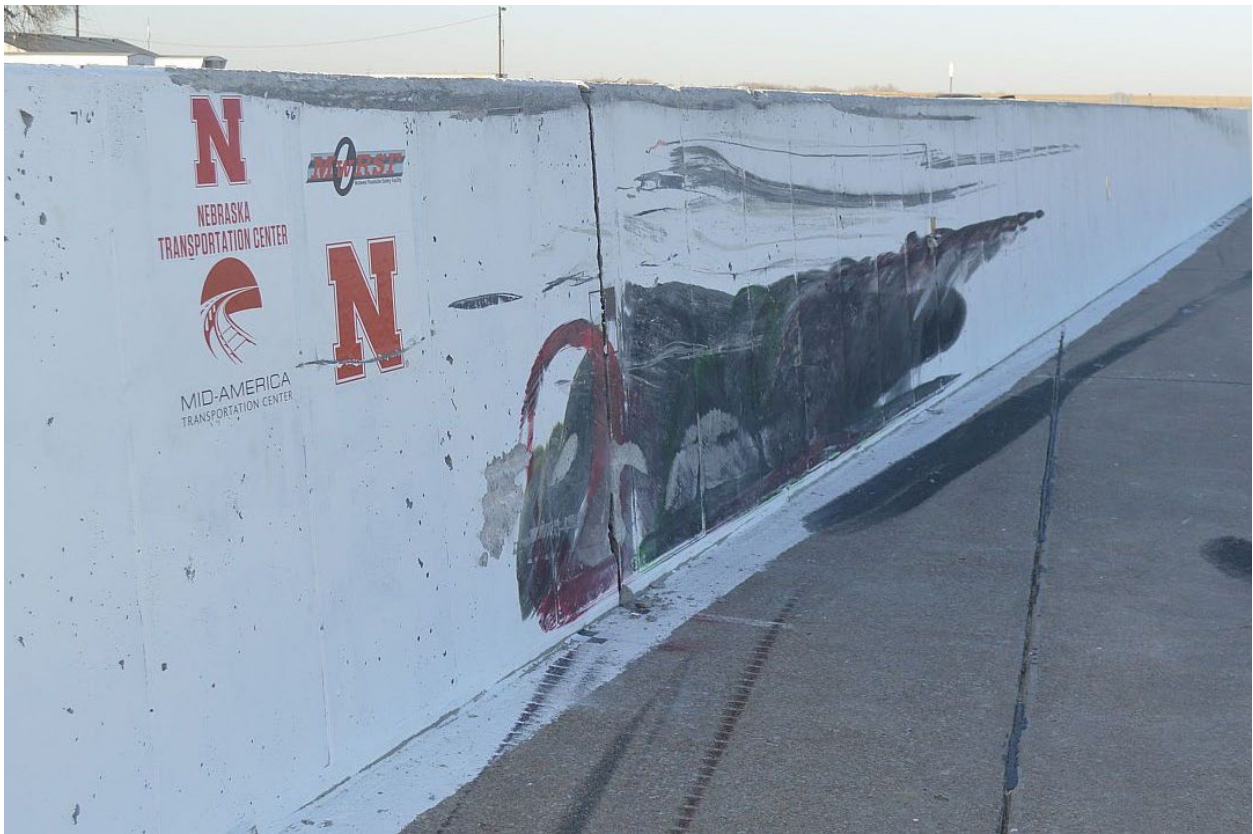
Figure 6.12 System Damage, Test No. MTL6-1
