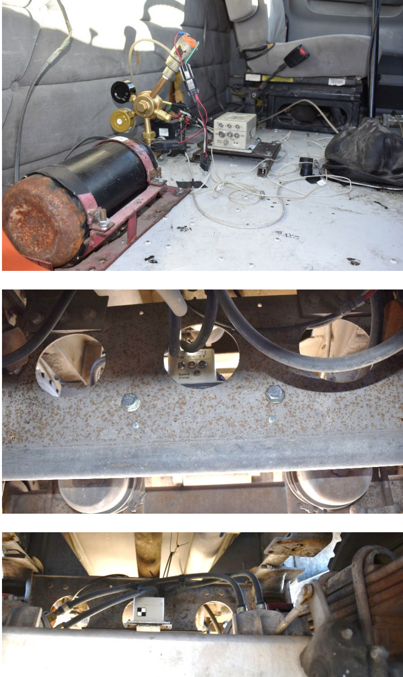
Figure 5.15 Accelerometer Mounting Locations, Test No. MTL6-1
