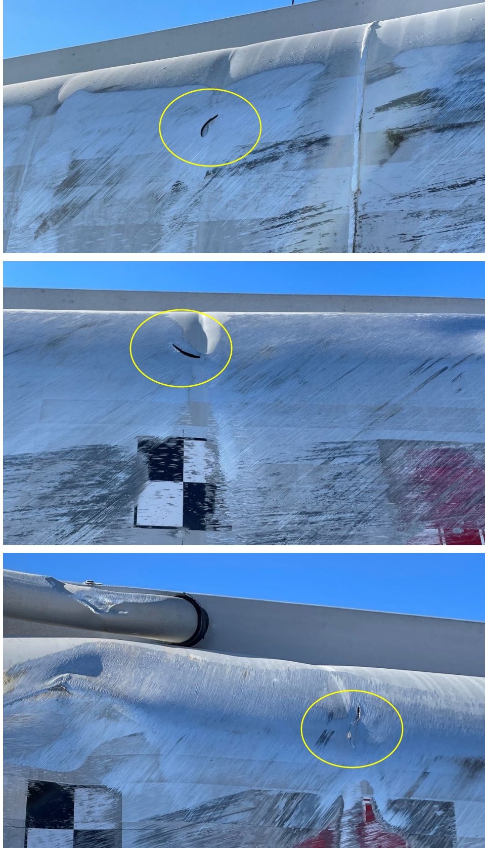
Figure 6.29 Tears in Trailer Jacket on Non-Impact Side, Test No. MTL6-1 109
