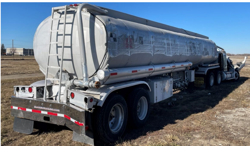
Figure 6.25 Trailer Damage After Uprighting, Test No. MTL6-1
