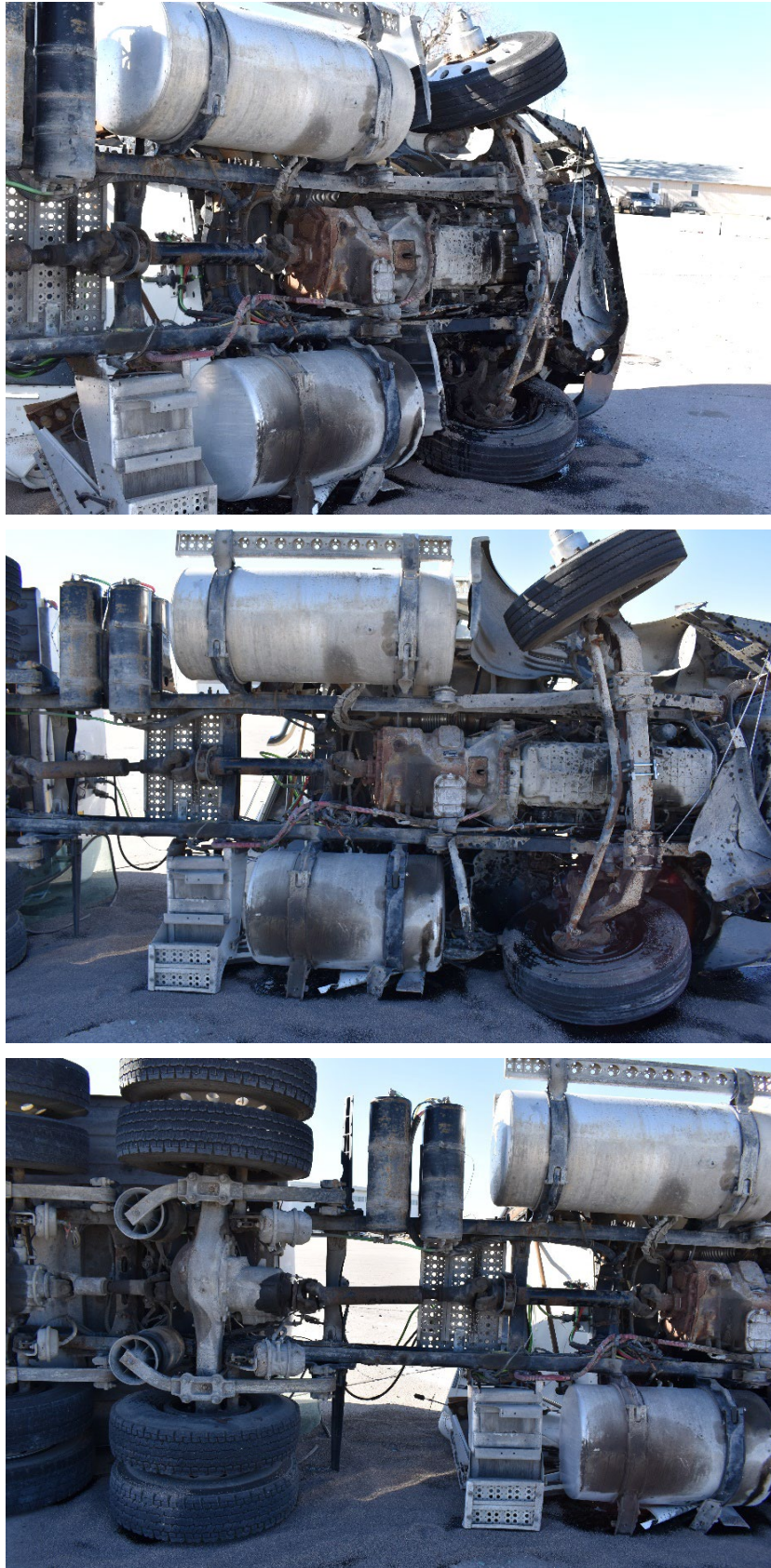
Figure 6.20 Tractor Undercarriage Chassis Damage, Test No. MTL6-1
