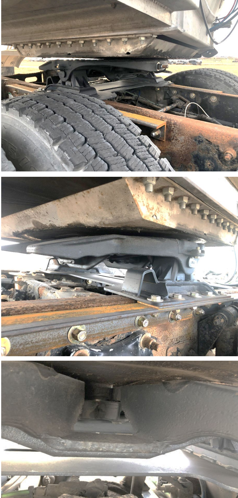
Figure 6.30 Fifth Wheel Damage, Test No. MTL6-1
