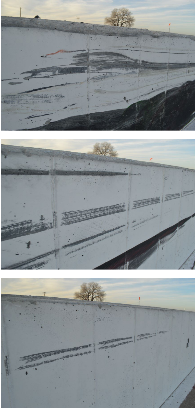
Figure 6.15 Scraping Damage along Top Impact-Side Edge of Barrier, Test No. MTL6-1
