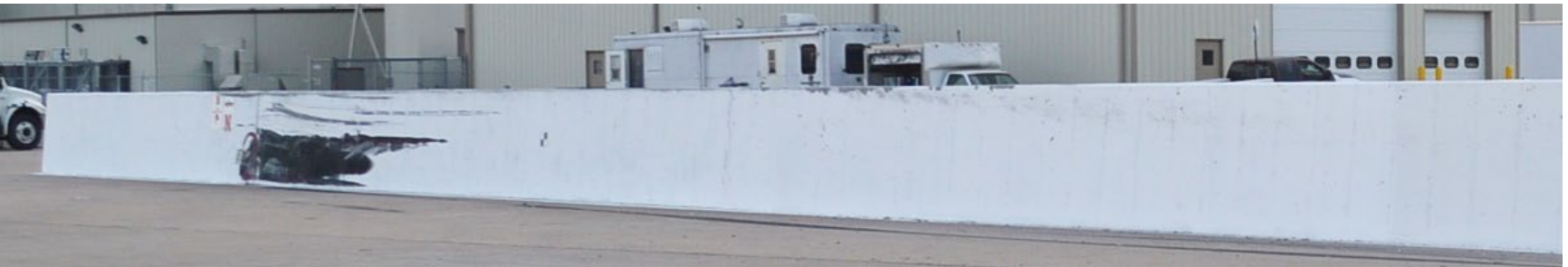
Figure 6.11 System Damage, Test No. MTL6-1
