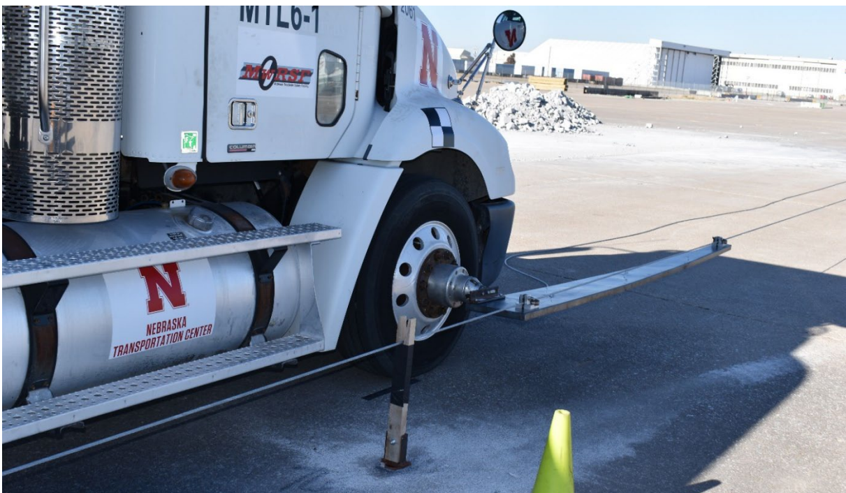
Figure 5.2 Test Vehicle Guidance System, Test No. MTL6-1
