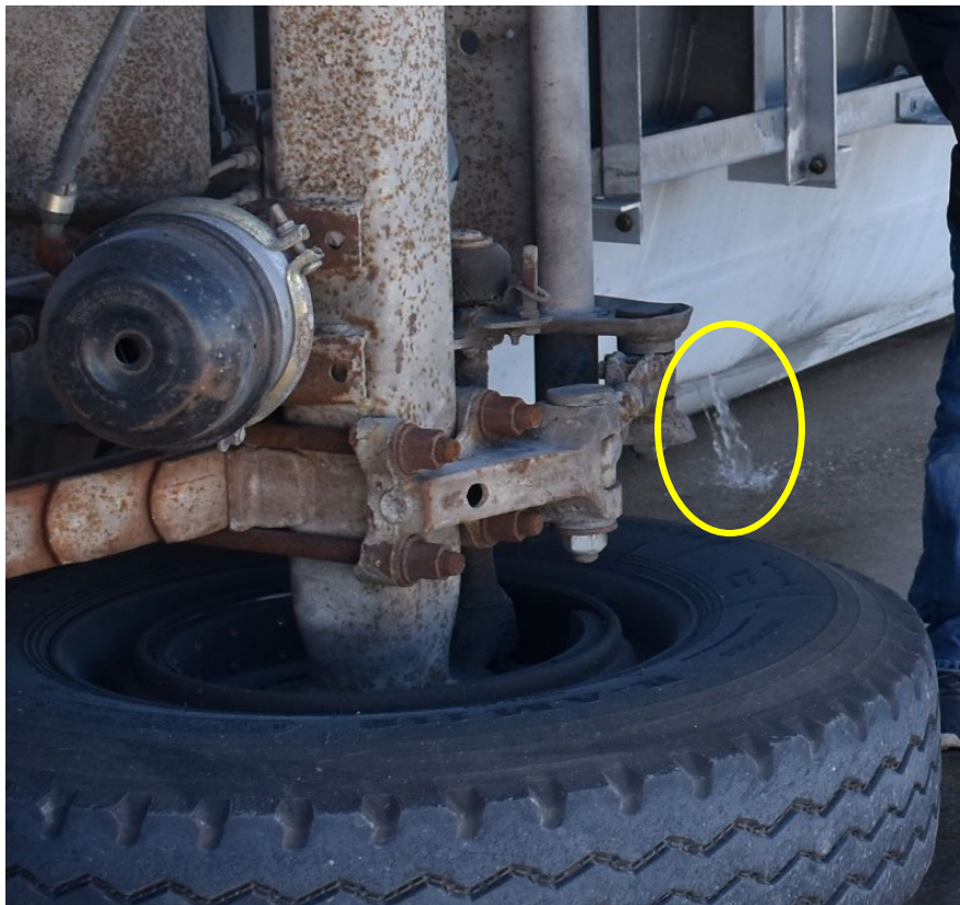
Figure 6.24 Locations of Trailer Leaks, Test No. MTL6-1
