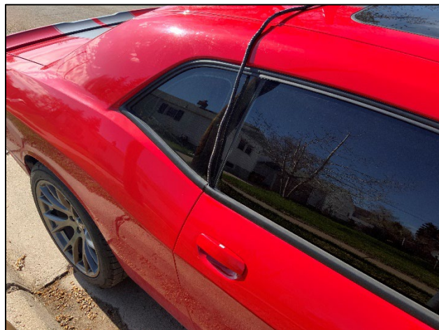
Step 5: Route the cables through the door frame so they are not pinched.
