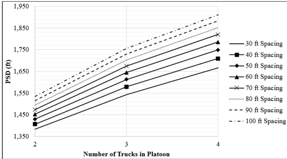
Figure 5.1 Computed passing sight distances for overtaking oil and gas truck platoons on a 70-mph two-lane highway. Source: Haq et al. (2021) (31).
