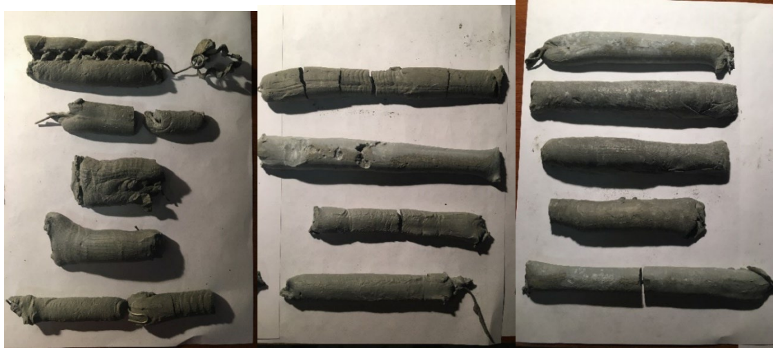
Figure 3.13 Printed Concrete Bars w/ Spiral Reinforcement Extrusion Variation.
