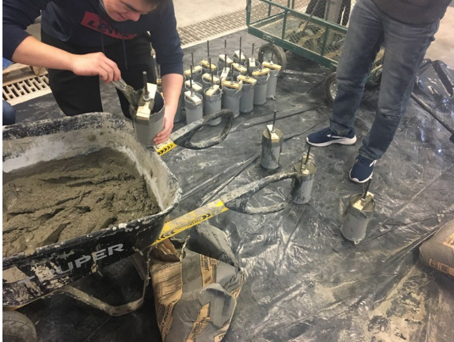
Figure 3.16 Manual Filling During Pour.
