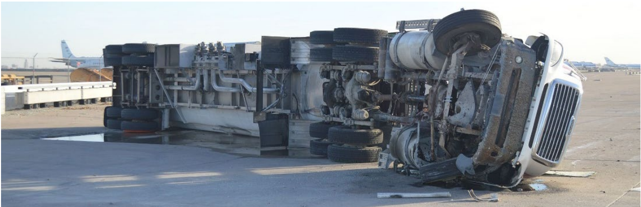
Figure 3.7 System and Vehicle Damage, Test No. MTL6-1
