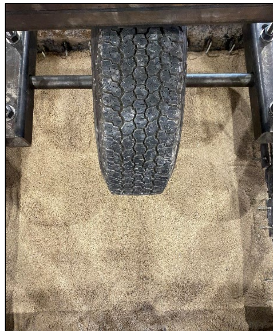
Figure 3.8 Compacted sand subgrade layer.
