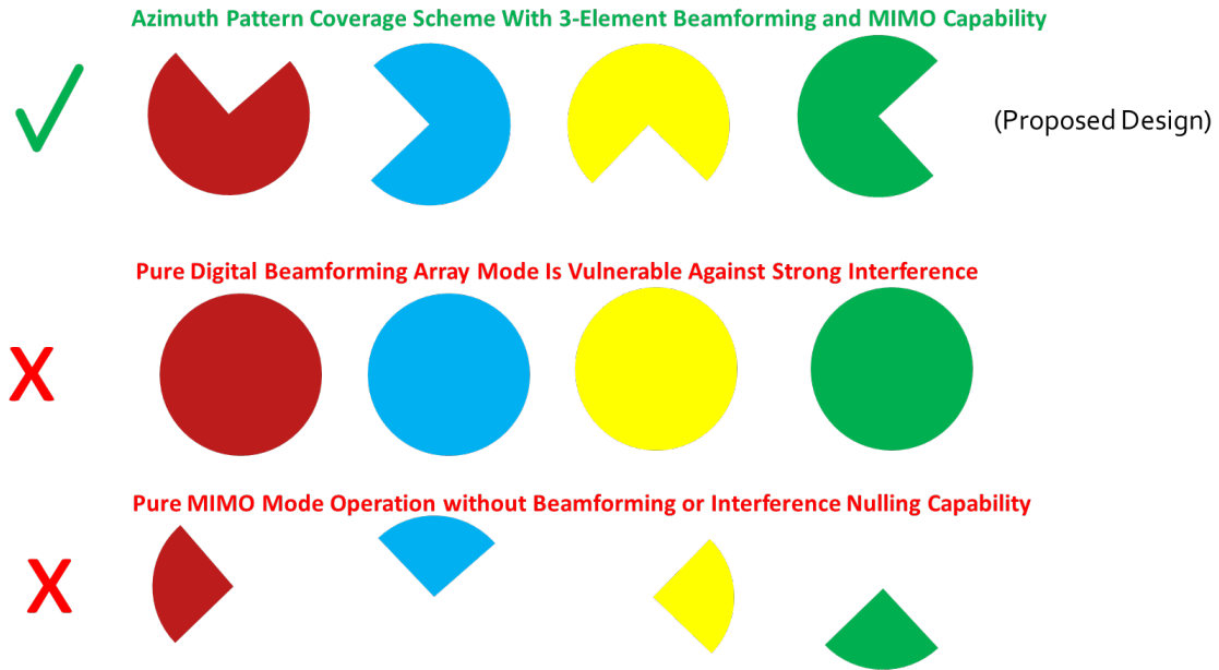
Figure 2 Different smart antenna system azimuthal pattern design approaches. (Top) proposed design (Middle) Beamforming Array Approach (Bottom) Pattern Diversity MIMO Approach
