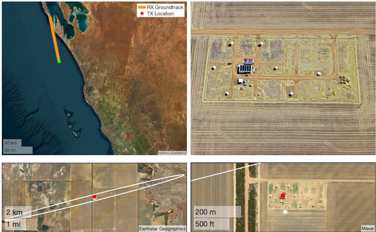
Fig. 3: Top: Experimental setup. The groundtrack of the LEO-based receiver is shown as well as the transmission site. Bottom: Final spoofer position estimate (white) using \gamma(t) . Shown in red is the true spoofer location. The error of the final estimate is 68 m. The emitter is contained within the 95% error ellipse, which has a semi-major of 6.7 km.
