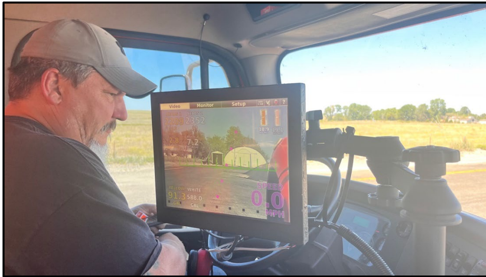
Figure 2.6: Monitoring Screen to Align Centerline
