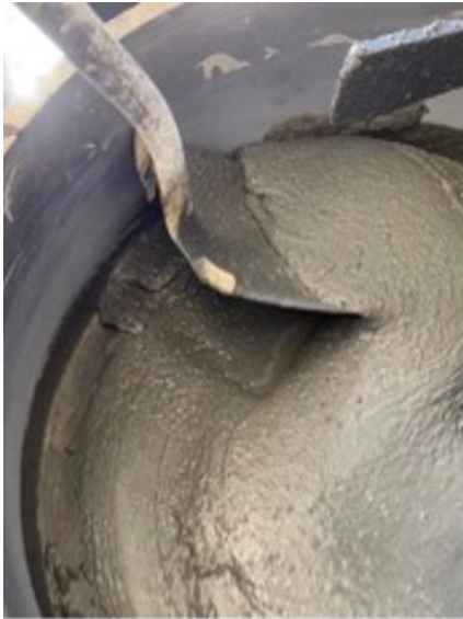
Figure 3.6: Mixture after Adding HRWR
