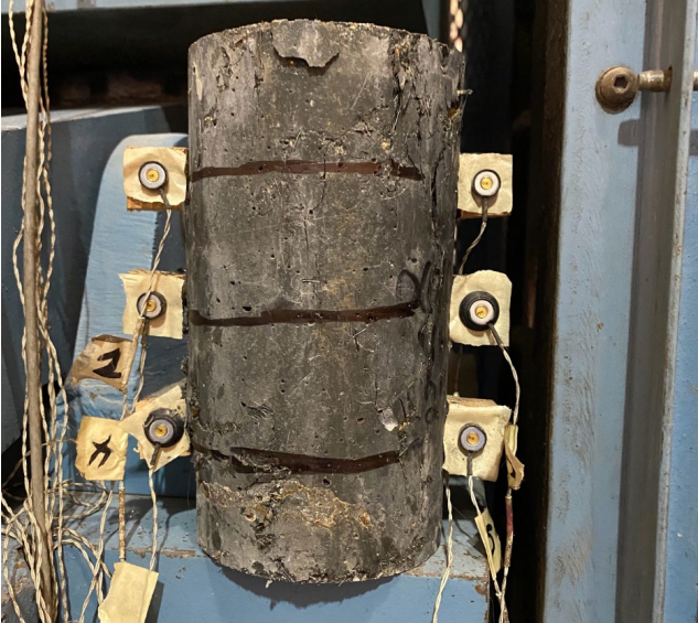
Figure 3.8: Marker Placement on Cylinder
