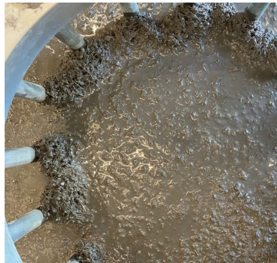
Figure 4.2: J-ring Test of Batch B16–LWA30%, with clear evidence of segregation/blocking of the fibers at the inner perimeter of the J-ring
