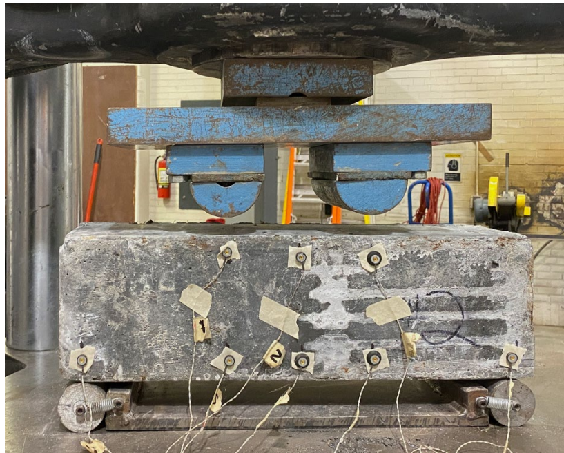
Figure 3.12: Beam Specimen with Eight Markers
