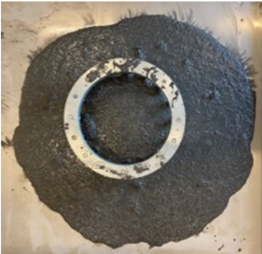
Figure 4.1: J-ring Test of Batch B15–LWA15%
