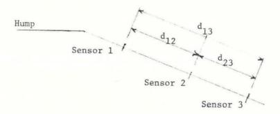
Placing sensors at three points along a uniform gradient of track will yield a time of arrival as a rail car passes. These times are represented at  $T_1$ ,  $T_2$ , and  $T_3$ . The distance between sensors 1, 2, and 3 are  $d_{12}$ ,  $d_{23}$  and  $d_{13}$ .
