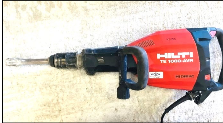
Figure 4.4 HILTI-TE 1000-AVR concrete jackhammer
