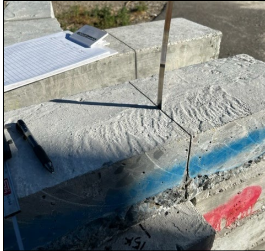
Figure 5.12 Measuring the line’s cutting depth
