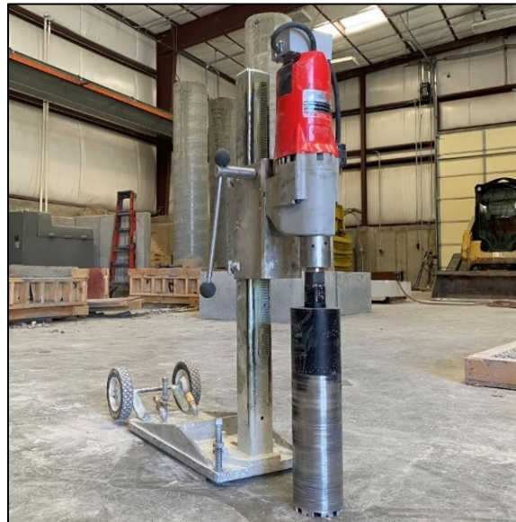
Figure 4.7 Concrete core test equipment
