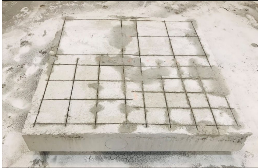
Figure 4.10 The concrete slab after saw cutting
