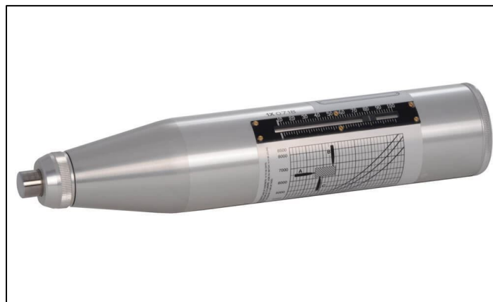
Figure 4.5 Gilson HM-705 Rebound hammer
