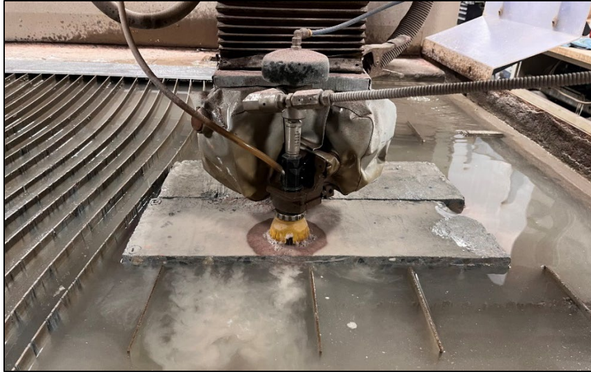
Figure 5.10 Penetration point cutting
