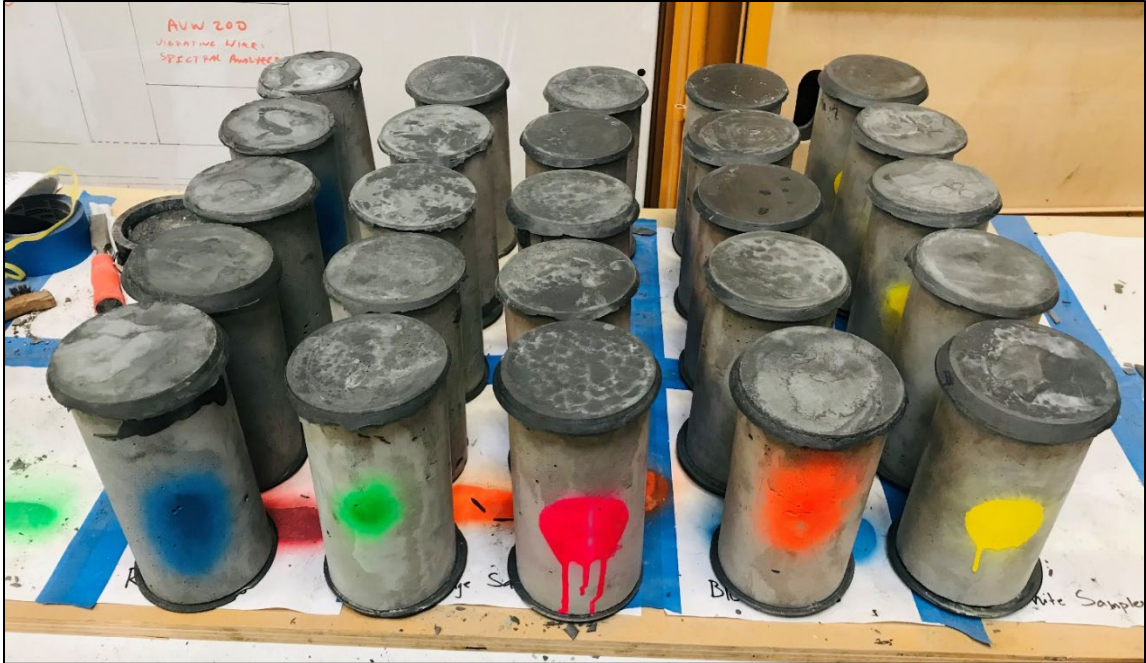
Figure 5.6 Cylinders for compressive strength
